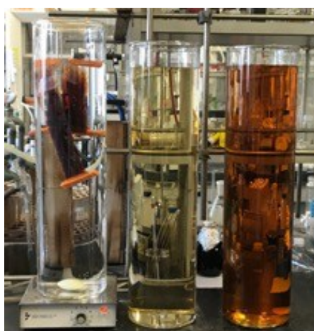
Figure S1. Digital image of the first (right), (b) second (middle), and (c) third (left) dialysis. The nanographenes smaller than the pore size of the given dialysis membrane leaked off from the membranes, while the larger ones remained in the membranes. The deionized waters became brown in the first dialysis, yellow in the second dialysis, and colorless in the third dialysis, indicating that the separation was finished. The three deionized waters (ca. 6 L each) were combined and concentrated. The resultant black aqueous solution was used in the next dialysis.
