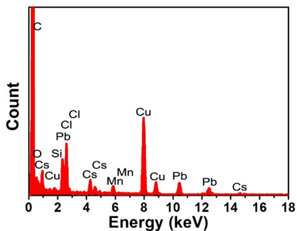
**Fig. S6** EDX spectrum of Mn-doped CsPbCl<sub>3</sub> NPLs prepared under a solvothermal reaction time of 4.5 h (with Mn-to-Pb feed ratio of 5:1).
