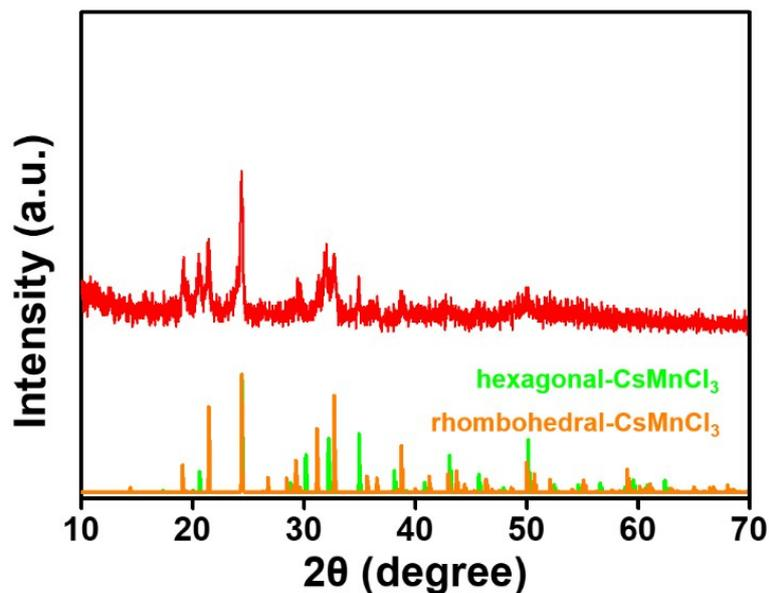
**Fig. S4** XRD pattern of the sample prepared after a prolonged reaction time over 12 h (with a Mn-to-Pb molar feed ratio of 10:1), indicating that the host CsPbCl<sub>3</sub> structure was nearly destroyed and phase of CsMnCl<sub>3</sub> was precipitated instead.
