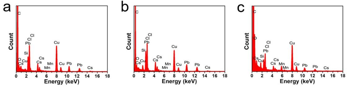
**Fig. S1** EDX spectra of Mn-doped CsPbCl<sub>3</sub> QDs prepared with different Mn-to-Pb molar feed ratios: (a) 5:1, (b) 7.5:1, and (c) 10:1. The compositions are CsPb<sub>0.94</sub>Mn<sub>0.06</sub>Cl<sub>3</sub>, CsPb<sub>0.85</sub>Mn<sub>0.15</sub>Cl<sub>3</sub> and CsPb<sub>0.75</sub>Mn<sub>0.25</sub>Cl<sub>3</sub>, respectively.
