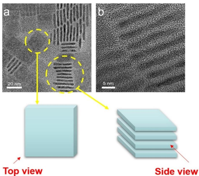
**Fig. S7** (a) TEM and (b) HRTEM image of ultrathin Mn-doped CsPbCl<sub>3</sub> NPLs with a thickness of 2 nm (using 3 mL of OA and OLA).
