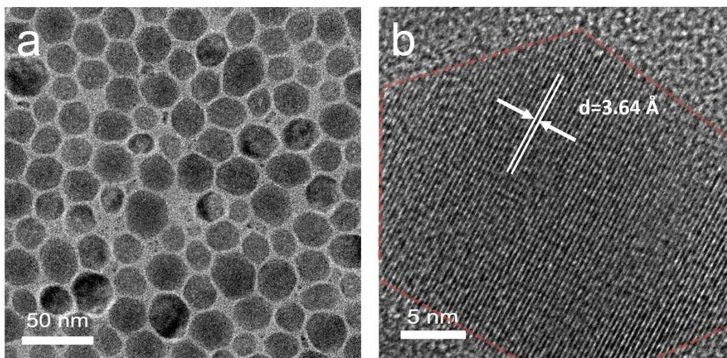
**Fig. S3** (a) TEM and (b) HRTEM image of CsMnCl<sub>3</sub> NCs formed by a spinodal decomposition process. The CsMnCl<sub>3</sub> NCs exhibit hexagon morphology with sizes of 16-32 nm. The interplanar lattice distance of 3.64 Å corresponds to the (104) plane of h-CsMnCl<sub>3</sub> or the (110) plane of r-CsMnCl<sub>3</sub>.
