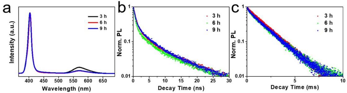
**Fig. S2** (a) Normalized PL spectra, (b) exciton PL lifetime and (c) Mn<sup>2+</sup> luminescence lifetime of Mn-doped CsPbCl<sub>3</sub> QDs prepared under different reaction times (with a same Mn-to-Pb molar feed ratio of 5:1 at 120 °C).
