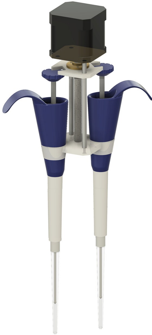
Figure S3. Potential design of the smart pipette which can hold and control two positive-displacement pipettes.
