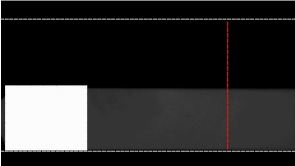
Movie S1. Flow-rate response of the OS pipette to pulse commands for a set flow rate of 97.4 \mu\text{L}/\text{min} . The set pulse widths were 0.5, 0.9, 2, 4, 8 and 12 seconds in order. The dotted red line denotes the ROI for interfacial position measurement.
