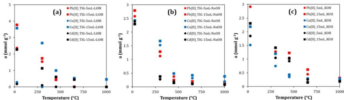
**Figure S5.** Dependence of adsorbed amount of Pb(II), Cu(II) and Cd(II) on annealing temperature of TIG-LiOH (a), TIG-NaOH (b) and TIG-KOH (c).
