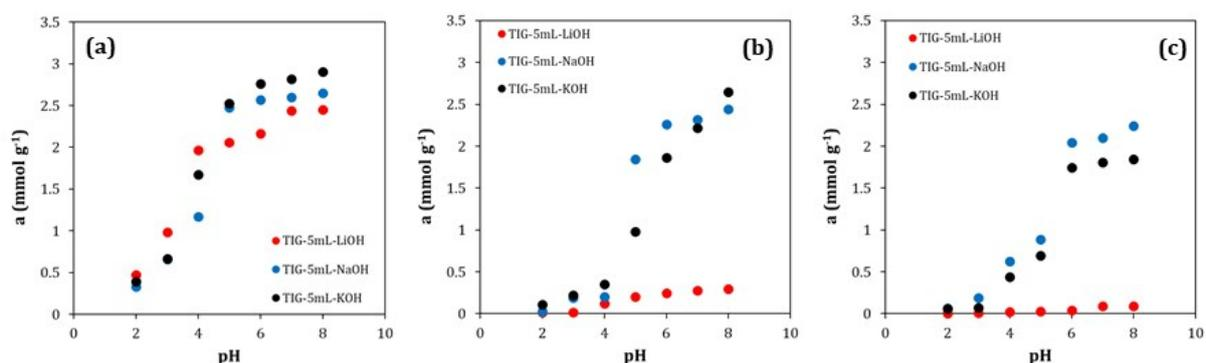
**Figure S4.** Dependence of pH on adsorbed amount of Pb(II) (a), Cu(II) (b) and Cd(II) (c) on of TIG-5mL-LiOH, TIG-5mL-NaOH and TIG-5mL-KOH.
