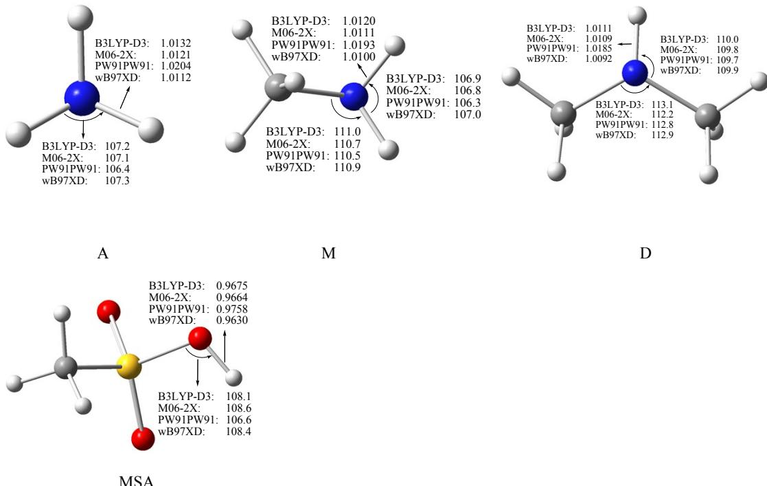
117 **Fig. S2** The optimized structures of dimers at the DFT/aug-cc-pVTZ (aug-cc-pV(T+d)Z for sulfur) level (angles in degrees; lengths in Å). The red, yellow, blue, gray, and white balls stand for O, S, N, C, and H atoms, respectively.
