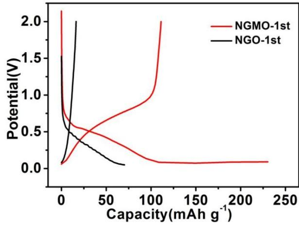
Fig. S3 The 1<sup>st</sup> discharged curves of NGMO and NGO.
