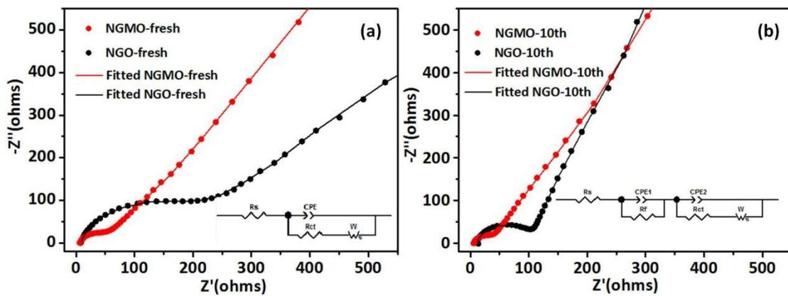
**Fig. S5** The fitting results of EIS, inside is the equivalent circuit model. NGMO and NGO (a) Fresh states, (b) 10th discharged cells.
