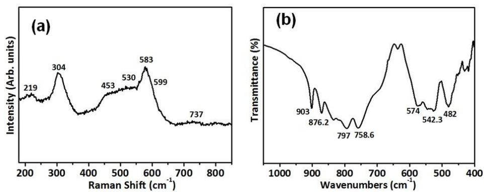
**Fig. S2** (a) Raman and (b) IR spectras of NGMO.
