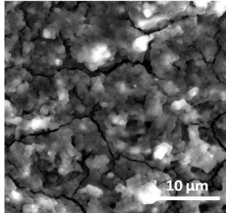
**Fig. S6** Long cycle performance and SEM image of discharged electrode of NGMO.
