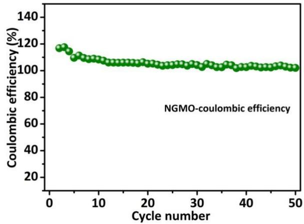
Fig. S4 The coulombic efficiency of NGMO in the first 50 cycles.
