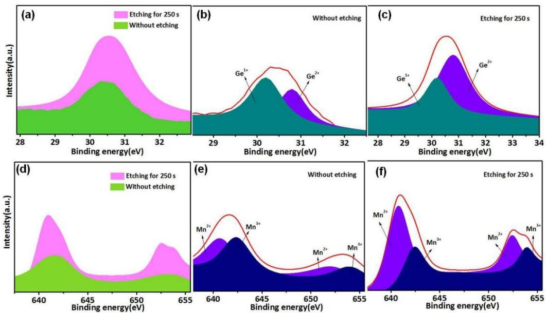
**Fig. S7** XPS spectra of 150<sup>th</sup> cycled electrode of NGMO without and with etching for 250 s by Ar plasma, (a) Ge 3d core level, (b) and (c) are the chemical valence states analysis of two electrodes, respectively. (d) Mn 2p core level, (e) and (f) are the chemical valence states analysis of two electrodes, respectively.
