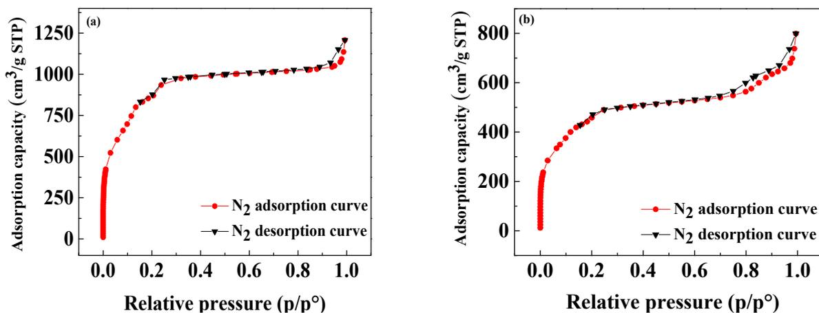
Fig S2. Nitrogen adsorption-desorption curves of Cr-MIL-101(a) and Fe-MIL-101-NH<sub>2</sub> (b)
