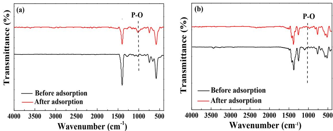
Fig S4. FT-IR spectra of Cr-MIL-101(a) and Fe-MIL-101-NH<sub>2</sub> (b) before and after TPhP adsorption
