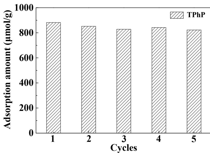
**Fig S9.** Adsorbed amounts of TPhP on the Cr-MIL-101 in five successive sorption cycles
