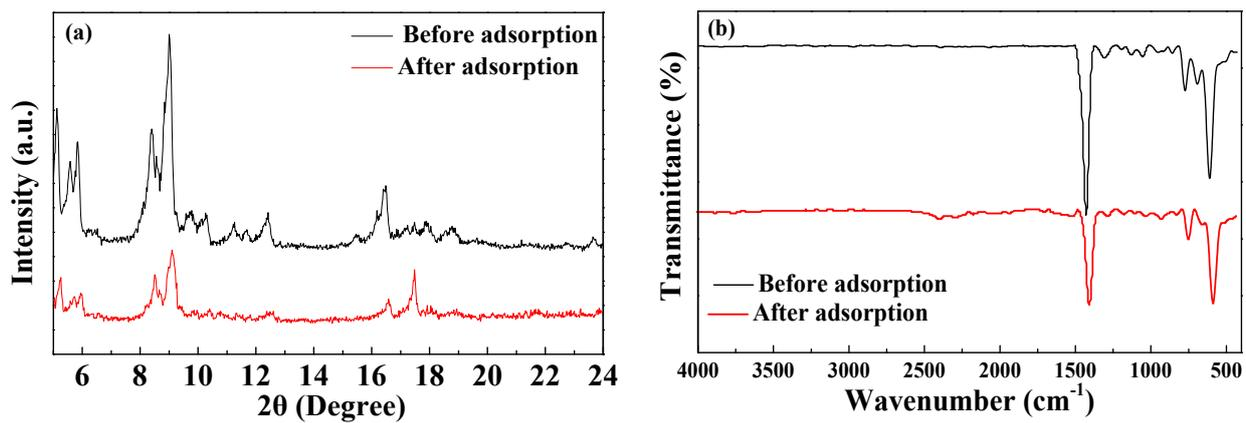
Fig S7. XRD patterns (a) and FTIR spectra (b) of Cr-MIL-101 before and after TPhP adsorption at pH 9
