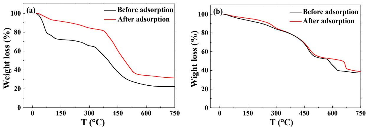
Fig S5. TGA curves of Cr-MIL-101(a) and Fe-MIL-101-NH<sub>2</sub> (b) before and after TPhP adsorption
