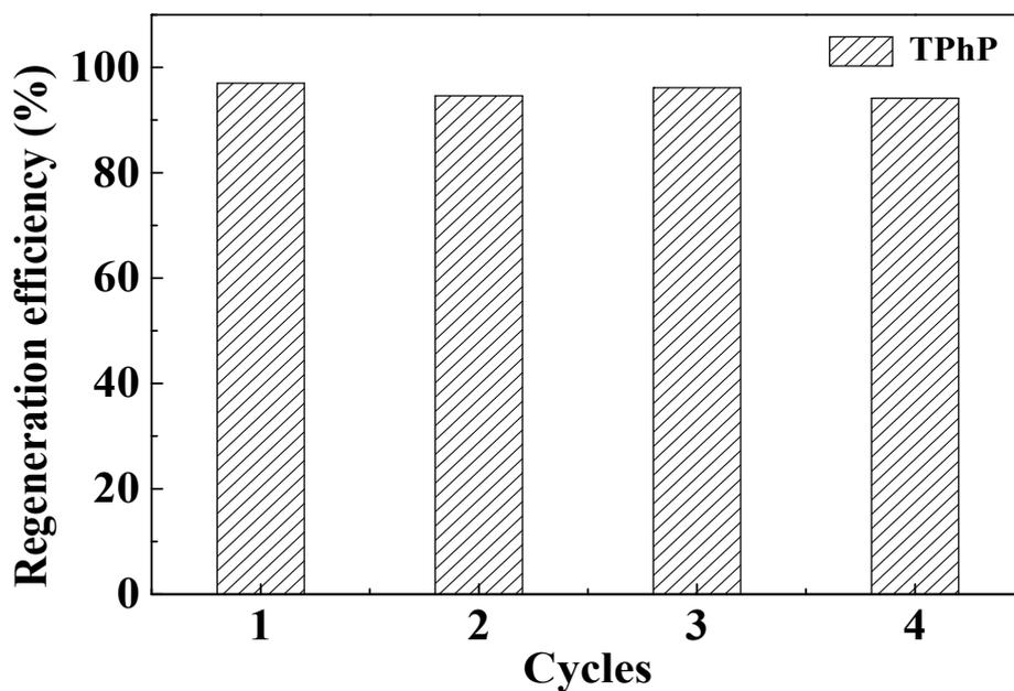
Fig S8. The regeneration efficiency of TPhP during successive sorption cycles
