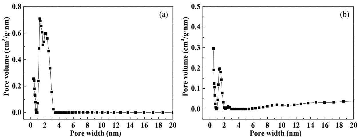
Fig S6. Pore size distribution of Cr-MIL-101(a) and Fe-MIL-101-NH<sub>2</sub> (b) after adsorption
