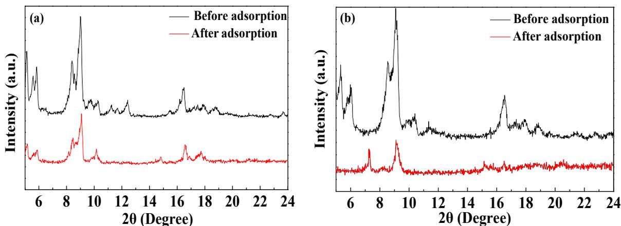
Fig S3. XRD patterns of Cr-MIL-101(a) and Fe-MIL-101-NH<sub>2</sub> (b) before and after TPhP adsorption
