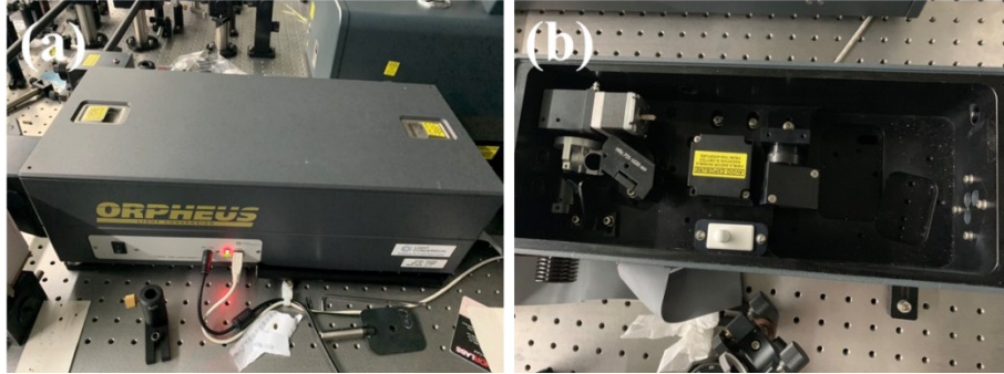
Figure S3 The optical parametric amplifier in femtosecond Z-scan measurement.
