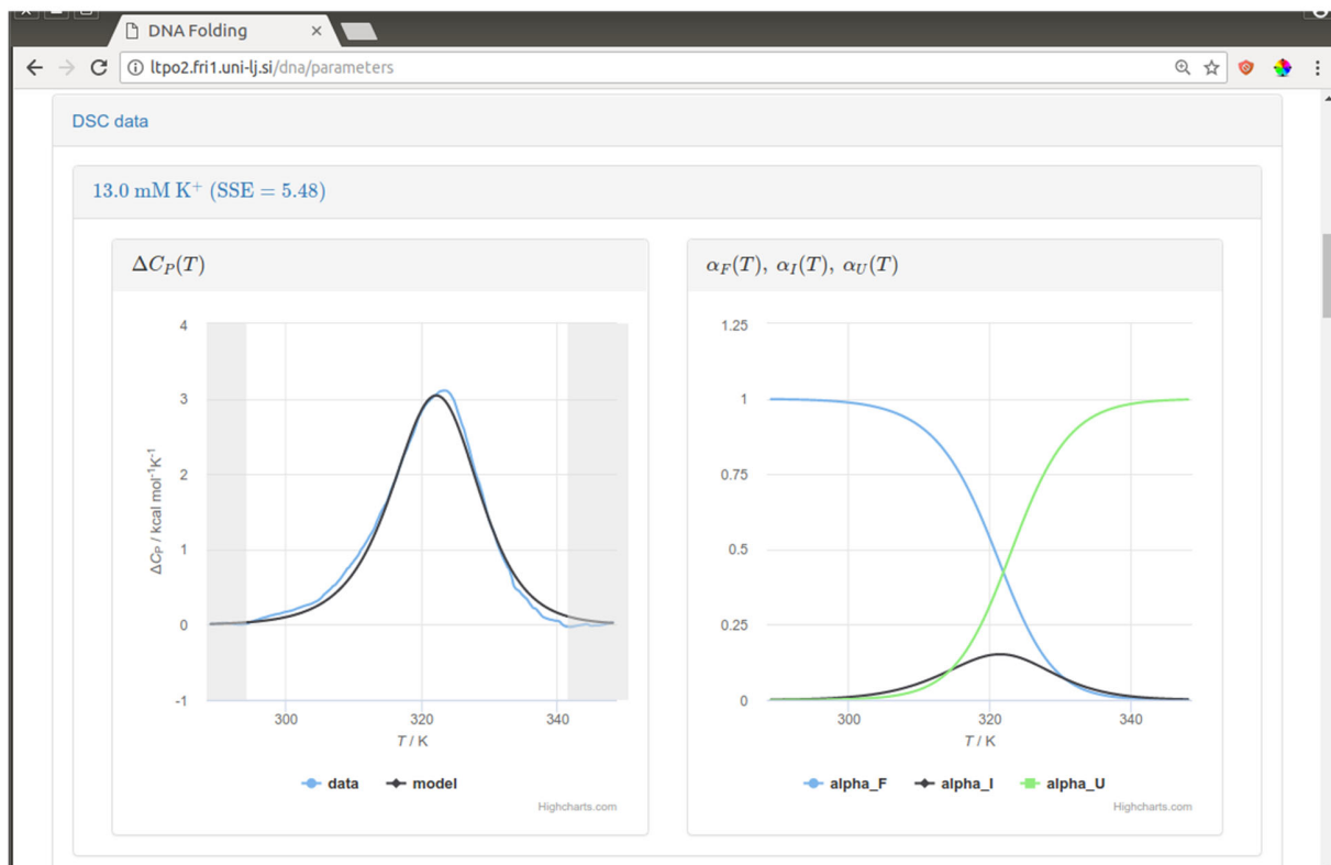
Fig. S4 Comparison of the fitting and experimental curves (left), and speciation diagram under the given conditions.
