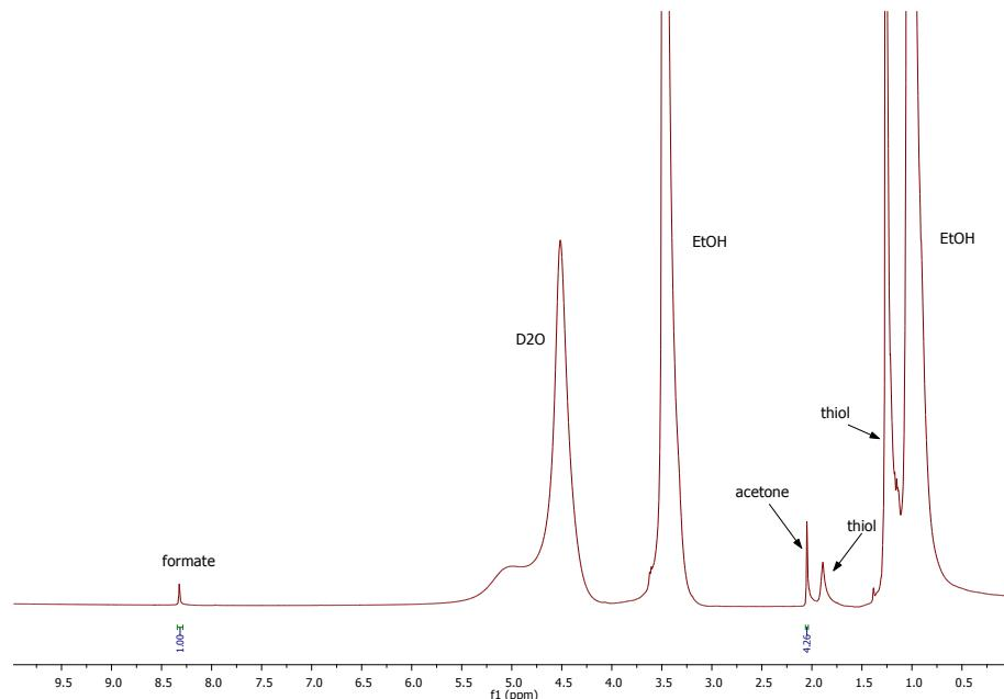
Figure S9: Catalysis in the presence of 2 methyl 2 propanethiol
