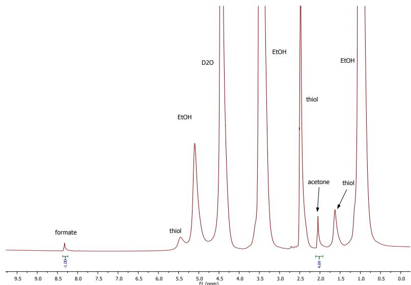
Figure S8 Catalysis in the presence of 2 mercapto-ethanol
