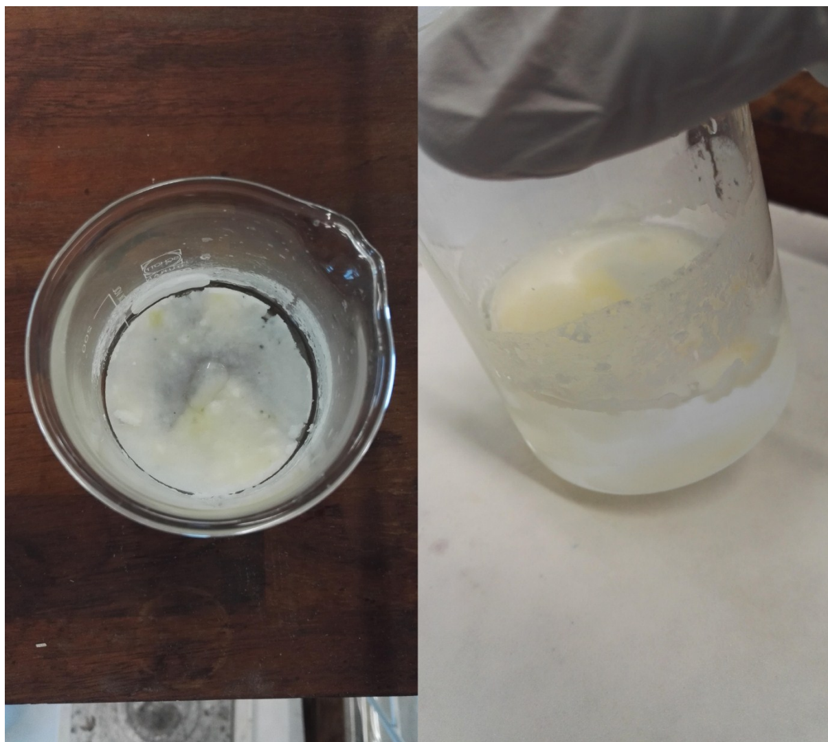
Figure S3: Photograph showing Compound 1 gelling thin 1-octadecene slicks ( ca. 2 mm thick) on deionised water.
