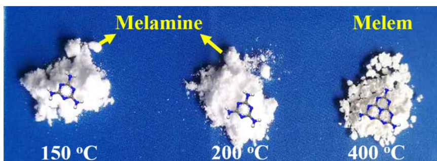
Figure S3 Photographs of the heated products of original melamine: remained \text{C}_3\text{N}_6\text{H}_6 at 150 °C and 200 °C, condensed into melem at 400 °C.
