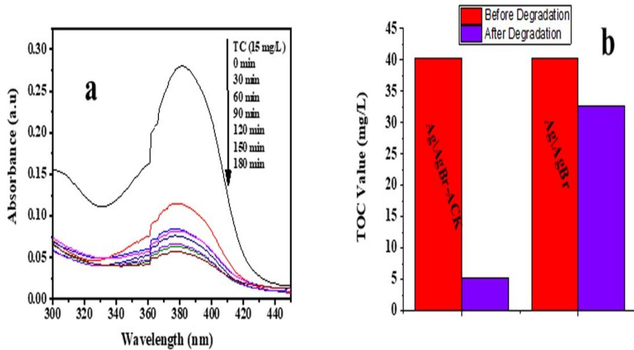
**Fig. S4.** (A) UV-Vis absorbance spectra of TC reduction in the presence of Ag-AgBr-ACK; (B) TOC reduction of TC using Ag/AgBr-ACK and Ag/AgBr catalyst.
