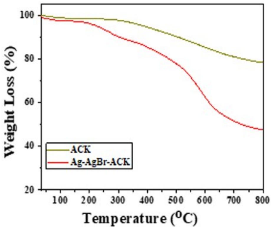
Fig. S3. TGA curves of ACK and Ag-AgBr-ACK
