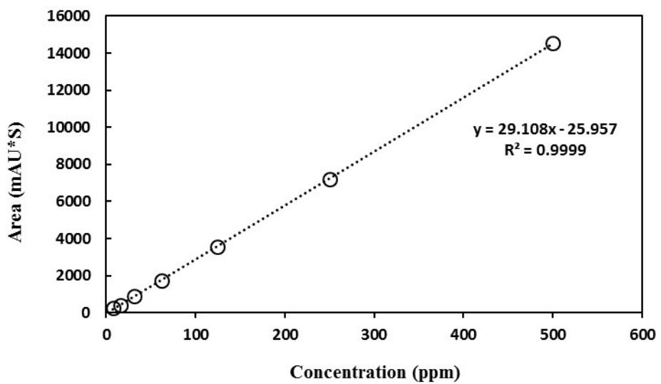
**Figure S1. (a) The HPLC curve of melatonin hormone at the concentration of 7.81 ppm and (b) the standard calibration curve for melatonin**
