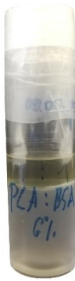
Fig. S11 – The two conjugated solutions obtained from the 6% blend (3% PLA, 3% BSA, 94% HFIP)
