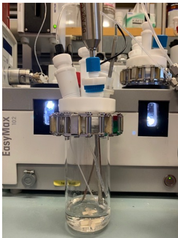
Figure S6. Photo of EasyMax reactor illustrating simultaneous ReactIR and automated sampling for crystallization analysis.
