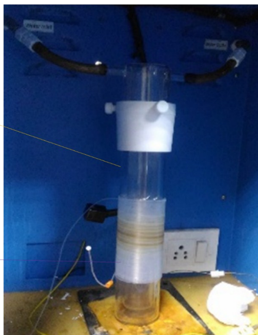
Figure S2: Basic set-up for photo-flow transfer hydrogenation reaction.
