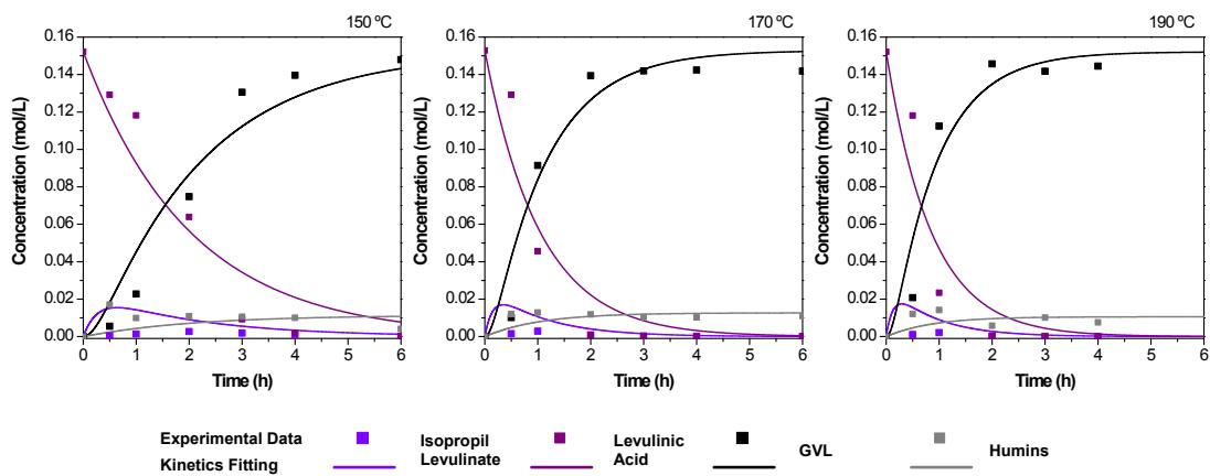
**Figure ESI 5.** Experimental (symbol) and modelled (solid lines) concentration of the compounds involved in the process of LA transformation into GVL in isopropanol over Zr-Al-Beta catalyst. Reaction conditions: temperature = 150 - 170 - 190 °C; catalyst loading = 12.5 g·L<sup>-1</sup>; levulinic acid concentration = 18 g·L<sup>-1</sup>; isopropanol volume = 0.04L.
