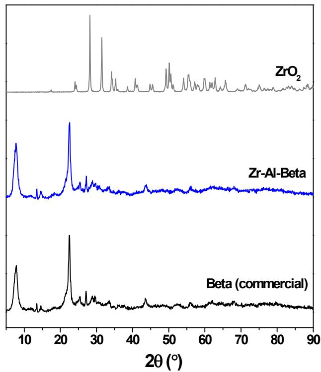
**Figure ESI 2.** XRD patterns of Zr-Al-Beta, as compared to commercial Beta zeolite and crystalline ZrO<sub>2</sub> (monoclinic phase).
