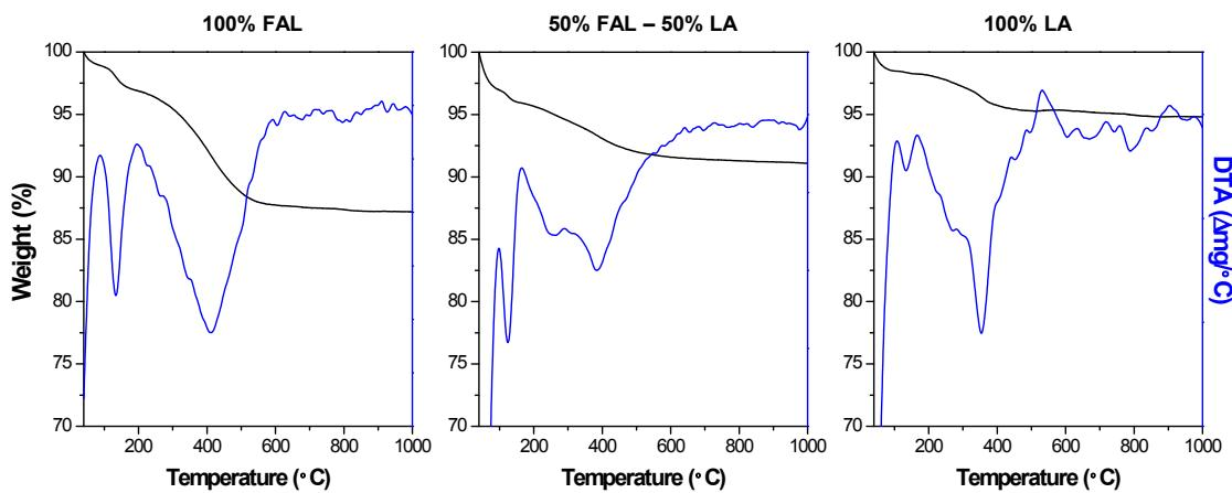
**Figure ESI 4.** Thermogravimetric analysis of spent Zr-Al-Beta used in the transformation of furfural (left), levulinic acid (right) and mixtures FAL-LA (50 % mol) (middle) into GVL. Reaction conditions: temperature = 170 °C; reaction time = 24 h, catalyst loading = 12.5 g·L<sup>-1</sup>; substrate concentration (FAL/LA) = 0.16 mol·L<sup>-1</sup>; isopropanol volume = 0.04L.
