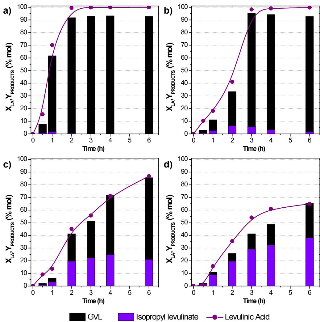
**Figure ESI 6.** Levulinic acid conversion and products distribution for the initial concentration study. Reaction conditions: temperature = 170 °C, catalyst loading = 12.5 g·L<sup>-1</sup>; levulinic acid concentration = (a) 18, (b) 63, (c) 152, (d) 300 g·L<sup>-1</sup>; isopropanol volume = 0.04 L.
