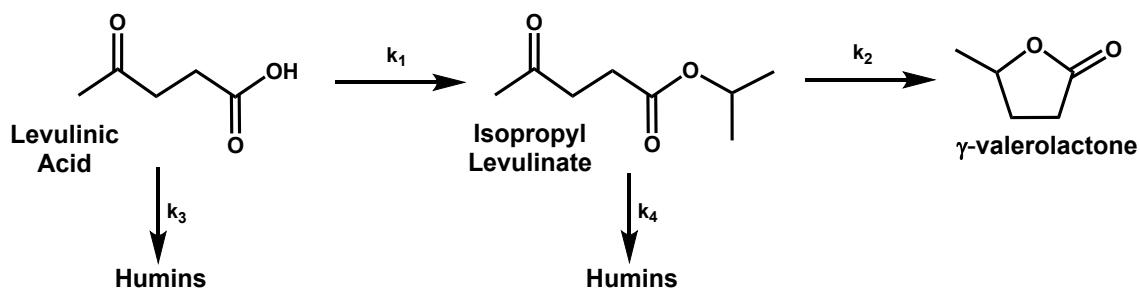
**Scheme ESI 1.** Proposed reaction network for the transformation of LA into GVL in isopropanol. Humins: degradation products.
