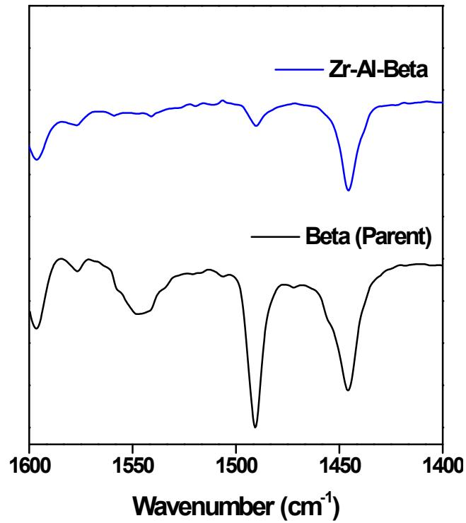
**Figure ESI 3.** DRIFT signals of adsorbed pyridine on parent (commercial) Beta and Zr-Al-Beta zeolites.
