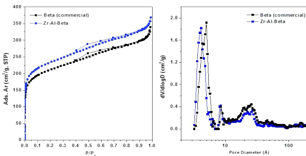
**Figure ESI 1.** Ar adsorption-desorption isotherms of commercial H-Beta zeolite and Zr-Al-Beta (left side). Pore sizes distribution of commercial H-Beta parent zeolite and Zr-Al-Beta (right side).
