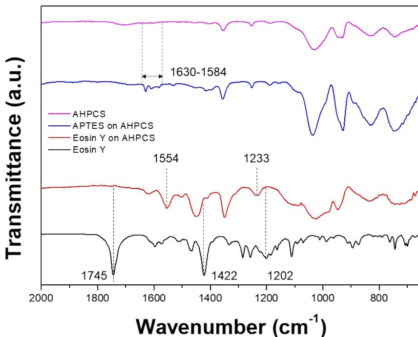
**Figure S2.** ATR-IR spectrum change by proceeding immobilization step.
