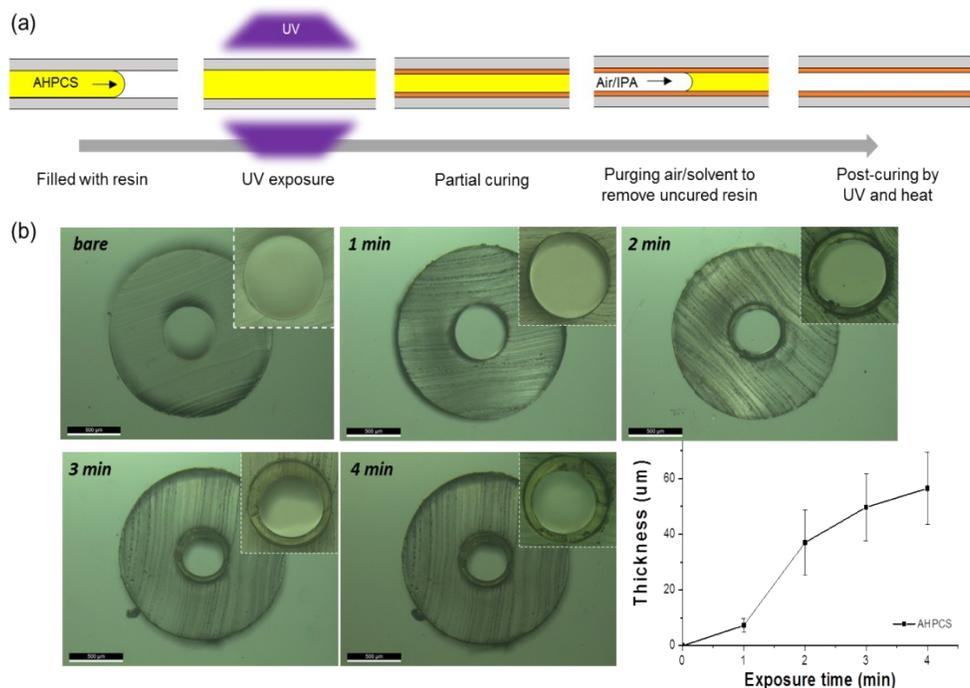
**Figure S1.** (a) Scheme for AHPCS coating into capillary tube, (b) cross-sectional optical images of AHPCS coated capillary tube, dependence of the coating thickness on UV exposure time.
