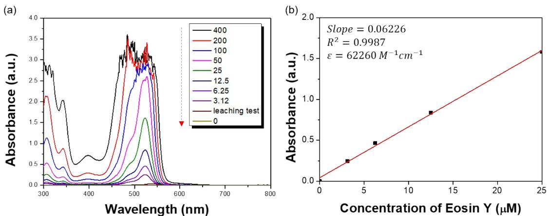
**Figure S4.** Eosin Y leaching test flowing solvent over a day. (a) UV-vis spectra of various concentration of the known concentration of Eosin Y, (b) calibration curve plot of absorbance at 523 nm versus concentration of Eosin Y.
