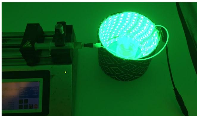
**Figure S3.** Experimental set-up of photocatalytic continuous-flow reaction in Eosin Y immobilized highly transparent perfluoroalkoxy alkane (HPFA) coil reactor with green LED.
