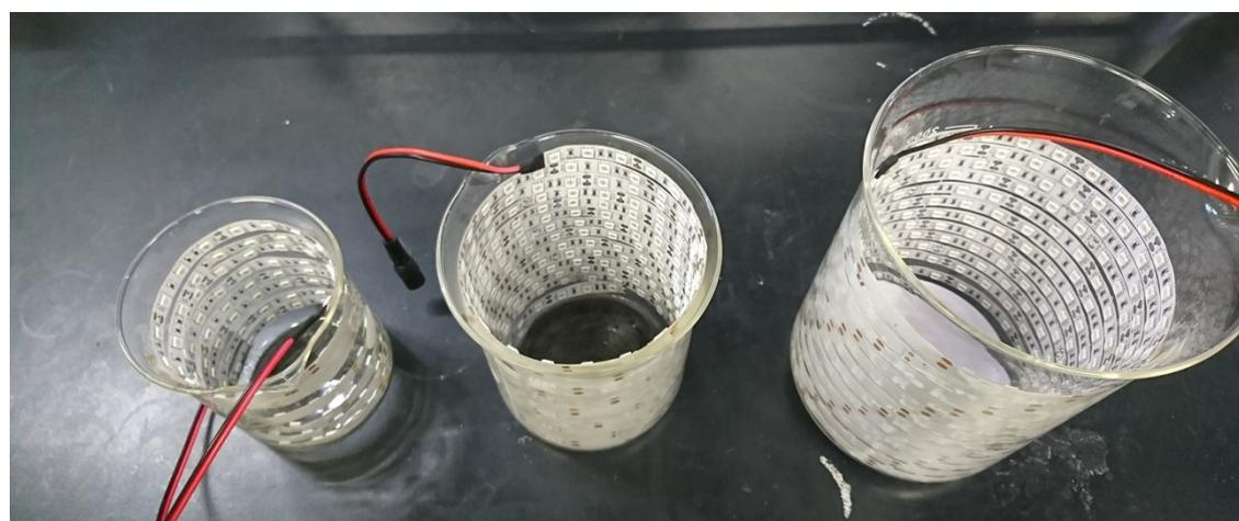
**Figure S1.** The light source of this reaction: 120 chips (left), 261 chips (middle), 297 tips (right).
