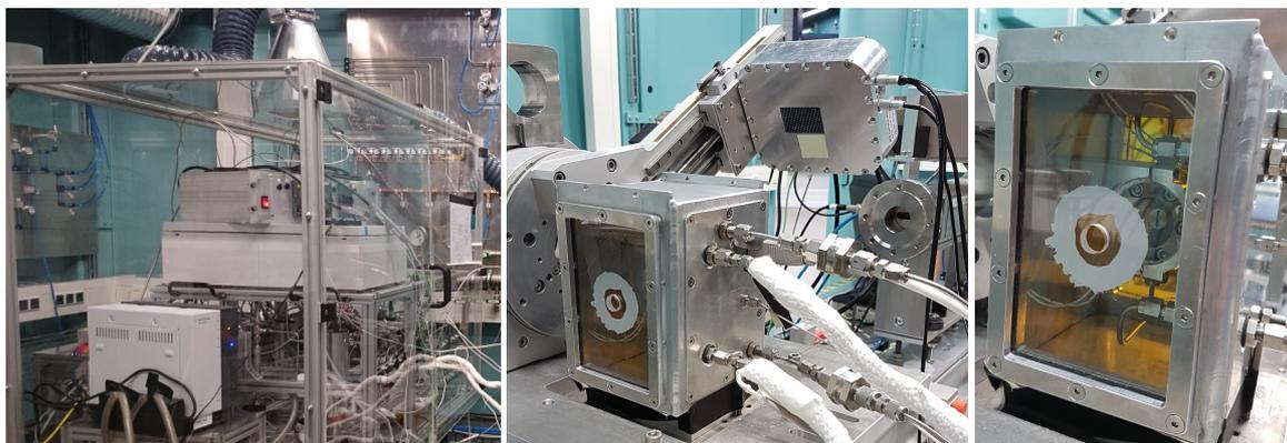
Figure S1: Pictures of the gas-dosing and -analysis unit (left), operando XAS&XRD setup (middle), high-pressure cell in safety box (c).
