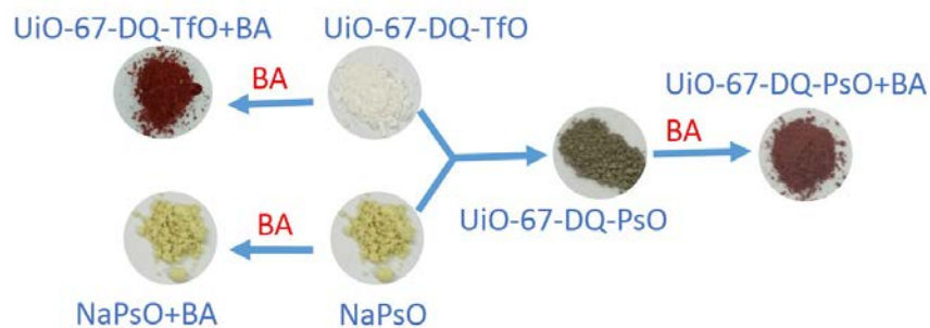
Fig. S8. Colors of NaPsO, UiO-67-DQ-TfO and UiO-67-DQ-PsO before and after exposure to butylamine (BA) vapor.
