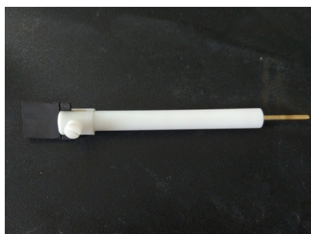
graphite plate electrode ( 15 \times 15 \times 2 \text{ mm}^3 )
