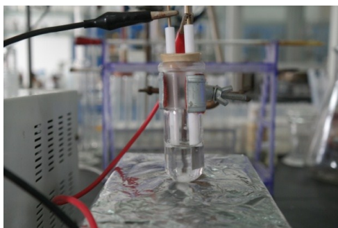
experiment apparatus (d: 24 mm, h: 80 mm)
