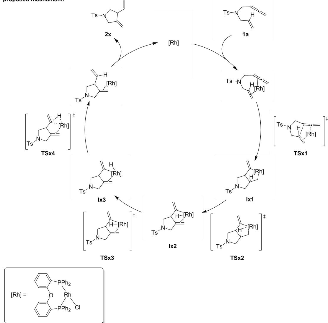
**Scheme S3** Proposed mechanism for Rh catalyzed cyclization of 1,6-allenes to the (not observed) five-membered product.
