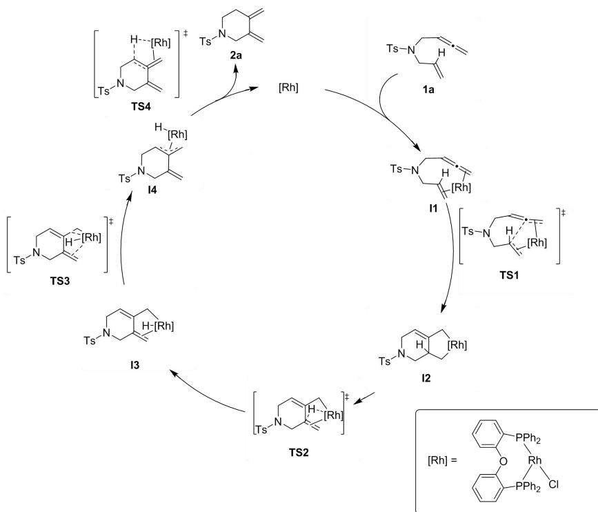
**Scheme S2.** Proposed mechanism for the Rh catalyzed cyclization of 1,6-allenes to six-membered exocyclic 1,3-dienes.
