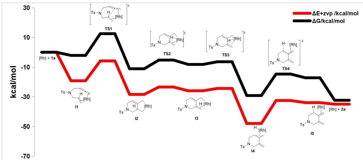
**Figure S1.** Computed catalytic cycle of the Rh catalyzed cyclization of 1,6-allenenes to six-membered exocyclic 1,3-dienes. All energies(PCM-M06/def2SVP//BP86/def2SVP) given with respect to energies of the [ClRh(DPEphos)] complex and the substrate.
