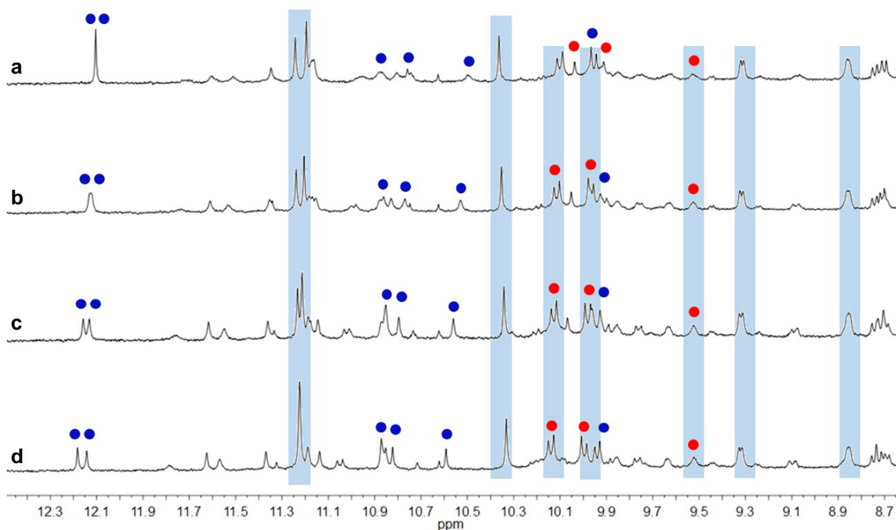
**Figure S9** Extract of <sup>1</sup>H NMR spectra (400 MHz, CDCl<sub>3</sub>) of **8b** at 55 °C (a), at 45 °C (b), at 35 °C (c) and 25 °C (d). Signals corresponding to the folded species are highlighted in blue. Red and blue dots indicate signals corresponding to OH protons.
