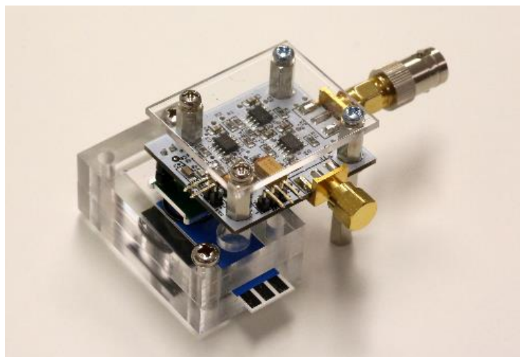
Figure S11. Photograph of the cell holder containing magnet and Zensor SPE, coupled with the silicon photomultiplier detector (ASD-RGB3S-P; AdvanSiD, Italy) and ASD-EP-EB-N amplifier board (AdvanSiD).
