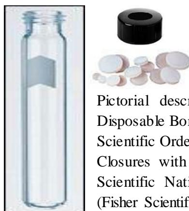
Pictorial description of reaction tube for *para*-olefination: Fisherbrand Disposable Borosilicate Glass Tubes (16\*125mm) with Threaded End (Fisher Scientific Order No. 1495935A) [left]; Kimble Black Phenolic Screw Thread Closures with Open Tops (Fisher Scientific Order No. 033407E); Thermo Scientific National PTFE/Silicone Septa for Sample Screw Thread Caps (Fisher Scientific Order No. 03394A).
