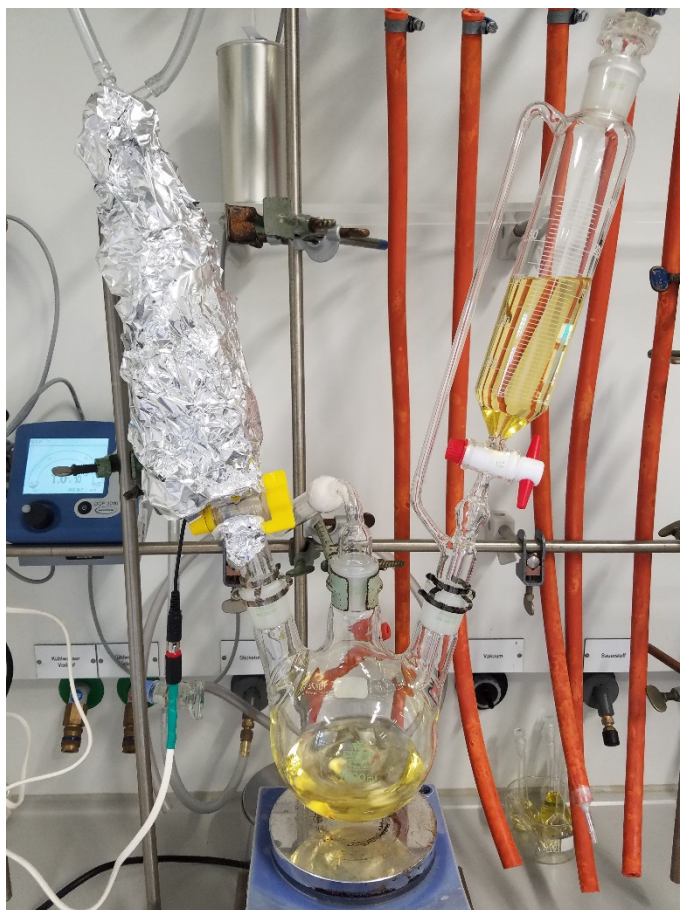
Figure S3: Macrocyclization setup for the synthesis of trisazo macrocycle 2.
