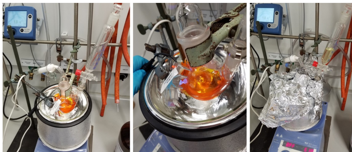
Figure S2: Macrocyclization setup for the synthesis of bisazo macrocycle 1 .
