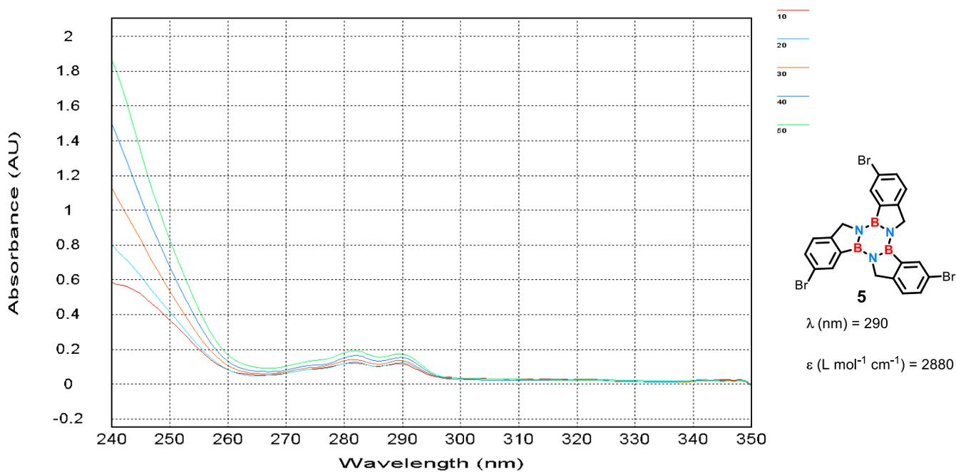
**Figure S13** | Variable Temperature Absorption spectra of borazine **5** in CHCl<sub>3</sub>
