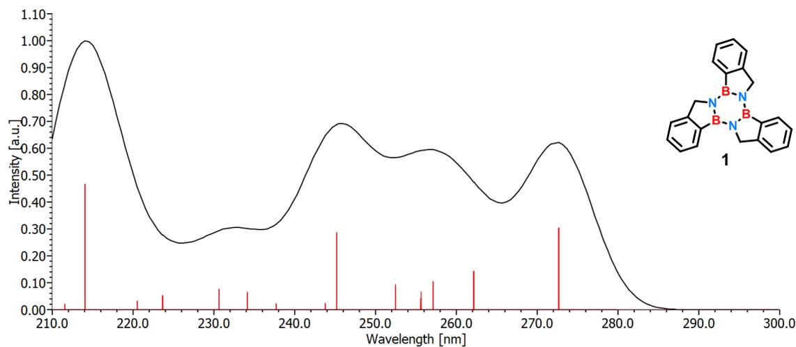
**Figure S21** | TD-DFT M11-L/6-311G(d,p) simulated UV-Vis spectra of borazine **1** in  $\text{CHCl}_3$
