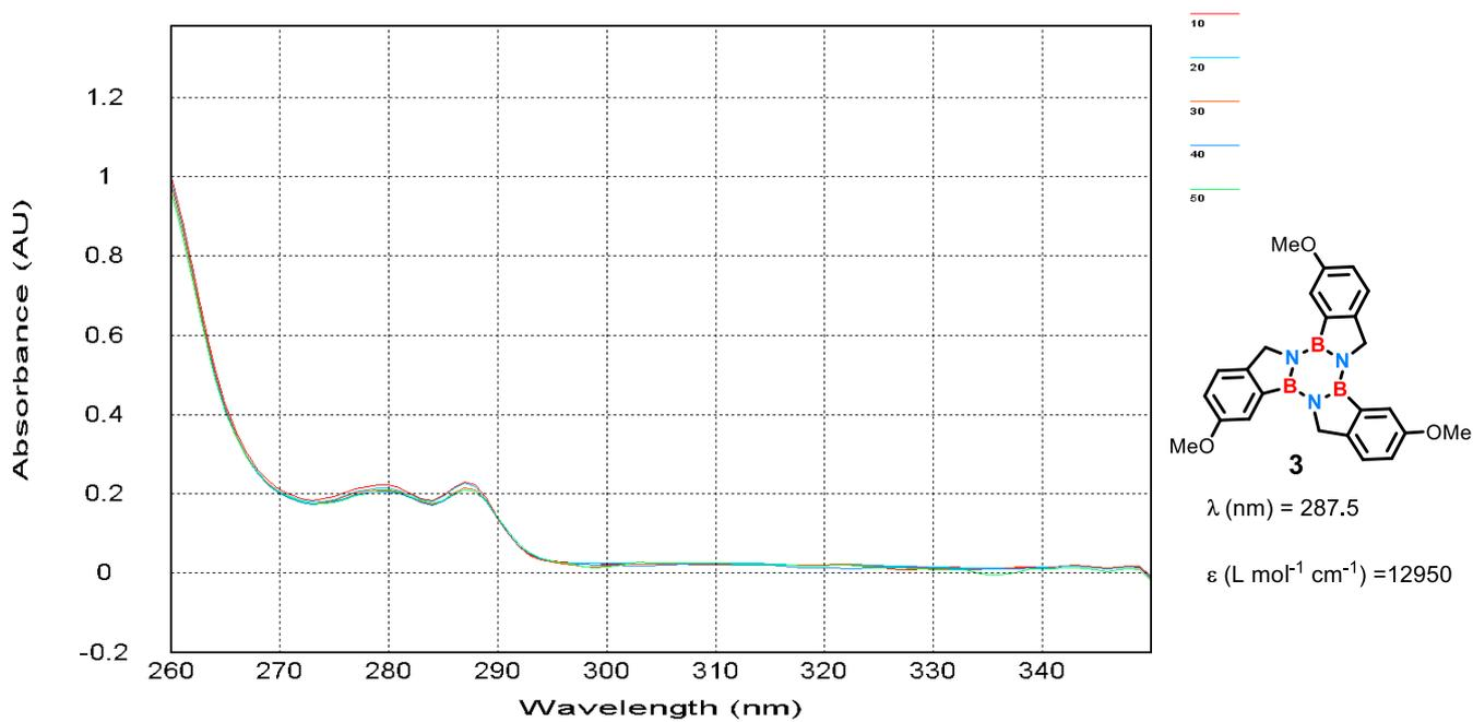
**Figure S12** | Variable Temperature Absorption spectra of borazine **3** in CHCl<sub>3</sub>
