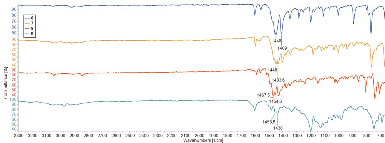
Figure S36. Stacked IR spectra of borazatruxenes 6, 7, 8 & 9.
