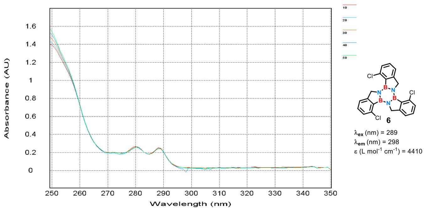
**Figure S14** | Variable Temperature Absorption spectra of borazine **6** in CHCl<sub>3</sub>
