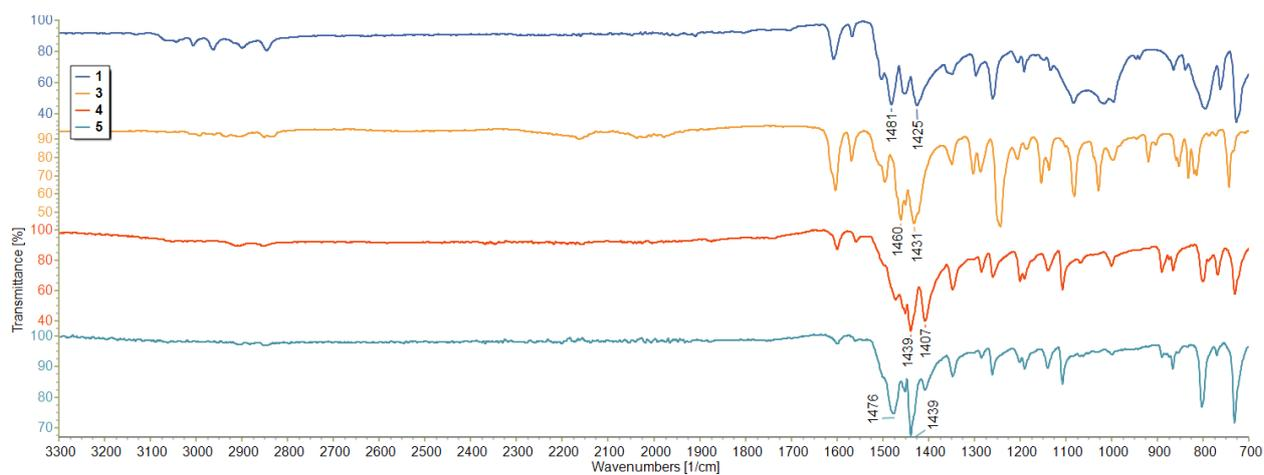
Figure S35. Stacked IR spectra of borazatruxenes 1, 3, 4 & 5.
