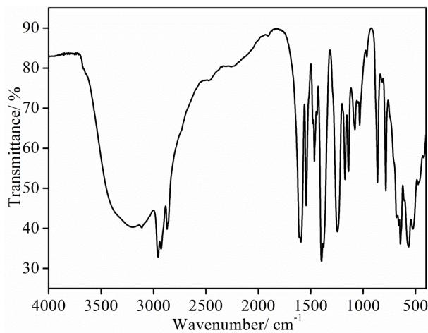
**Figure S21.** IR spectrum of compound **TOC-16**.
