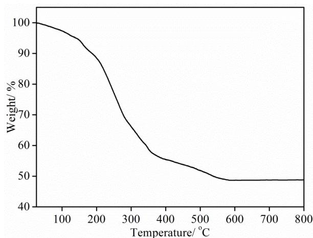
**Figure S27.** TG curve of compound **TOC-15** in  $\text{N}_2$  atmosphere.
