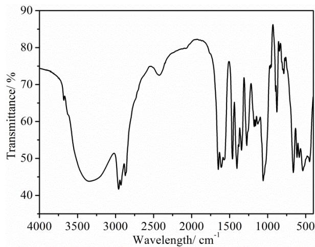
**Figure S19.** IR spectrum of compound **TOC-14**.
