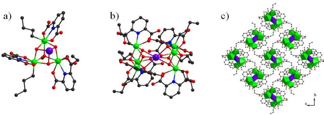
**Figure S1.** The asymmetric unit (a), cluster structure (b), and packing mode (c) of **TOC-12**. Atom color code: green Sn; purple Na; red O; black C; dark blue N. Polyhedral color code: green SnO<sub>5</sub>CN; purple NaO<sub>6</sub>.
