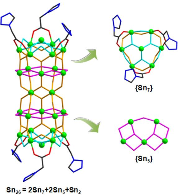
**Figure S4.** The ball-and-stick illustration of  $\text{Sn}_{26}$  cluster in **TOC-15**. Atom color code: green Sn.
