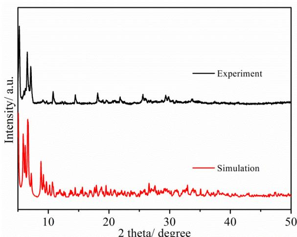
**Figure S15.** Simulated and experimental PXRD pattern of compound **TOC-17**.
