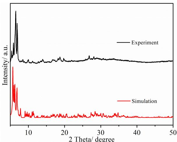
**Figure S14.** Simulated and experimental PXRD pattern of compound **TOC-16**.
