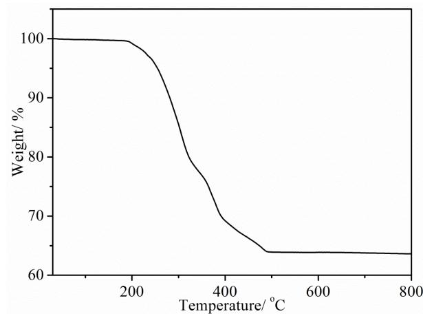
**Figure S30.** TG curve of compound **TOC-18** in N<sub>2</sub> atmosphere.
