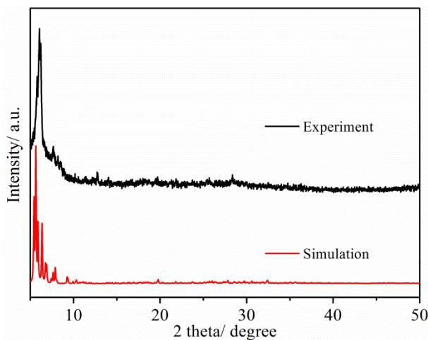
**Figure S13.** Simulated and experimental PXRD pattern of compound **TOC-15**.
