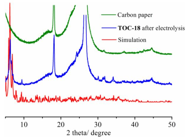
**Figure S47.** Simulated PXRD pattern of **TOC-18** and experimental PXRD patterns of carbon paper and **TOC-18** on carbon paper after electrocatalysis.
