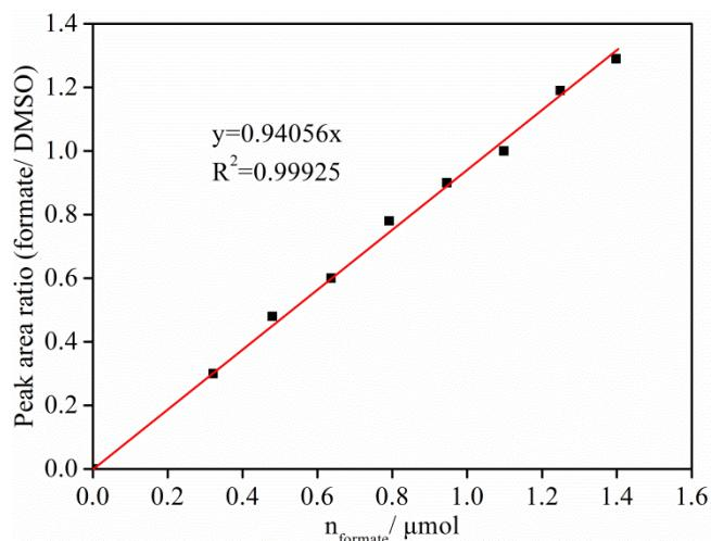
**Figure S44.** The calibration curve for formate (DMSO as internal standard).
