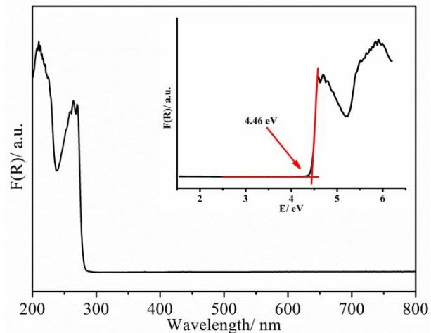
**Figure S32.** UV-vis diffuse reflectance spectrum of **TOC-13**.
