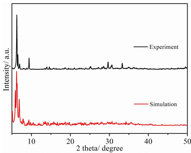
**Figure S16.** Simulated and experimental PXRD pattern of compound **TOC-18**.
