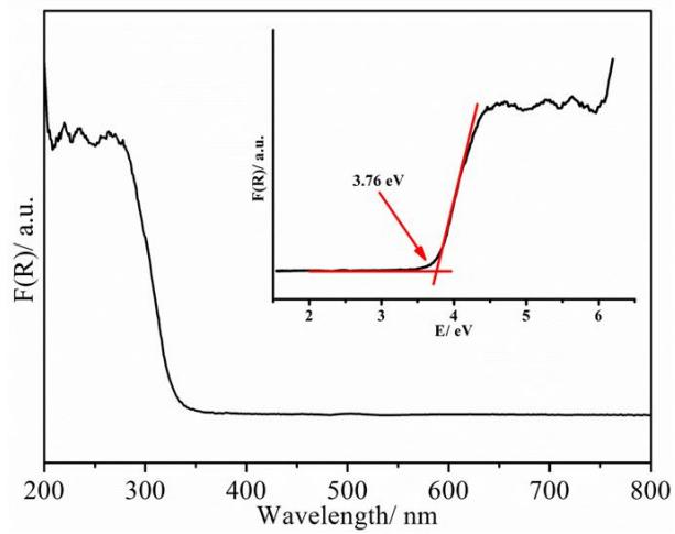
**Figure S31.** UV-vis diffuse reflectance spectrum of **TOC-12**.
