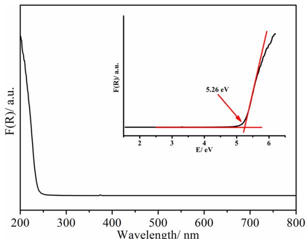
**Figure S33.** UV-vis diffuse reflectance spectrum of **TOC-14**.
