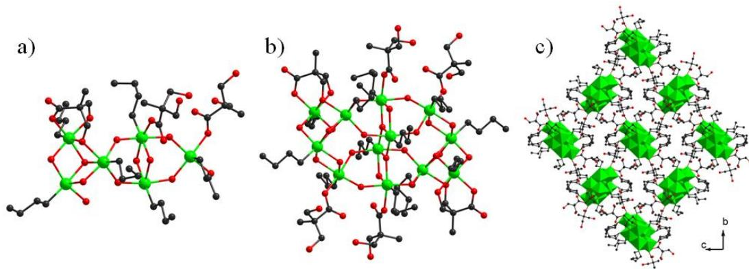
**Figure S3.** The asymmetric unit (a), cluster structure (b), and packing mode (c) of **TOC-14**. Atom color code: green Sn; red O; black C. Polyhedral color code: green SnO<sub>5</sub>C.
