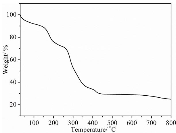
**Figure S26.** TG curve of compound **TOC-14** in  $\text{N}_2$  atmosphere.
