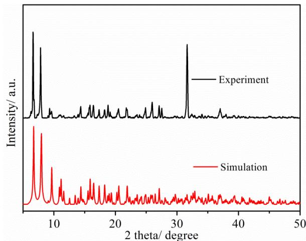
**Figure S11.** Simulated and experimental PXRD pattern of compound **TOC-13**.
