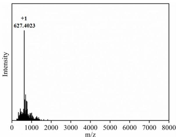
**Figure S43.** The positive-mode ESI-MS spectrum of mother liquor for **TOC-18** diluted by ethanol.
