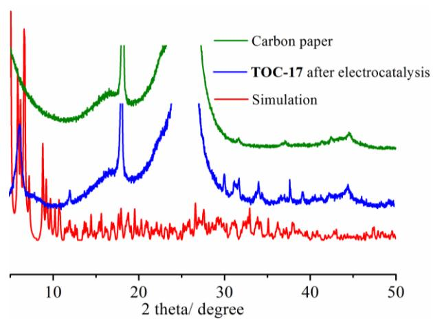
**Figure S46.** Simulated PXRD pattern of **TOC-17** and experimental PXRD patterns of carbon paper and **TOC-17** on carbon paper after electrocatalysis.
