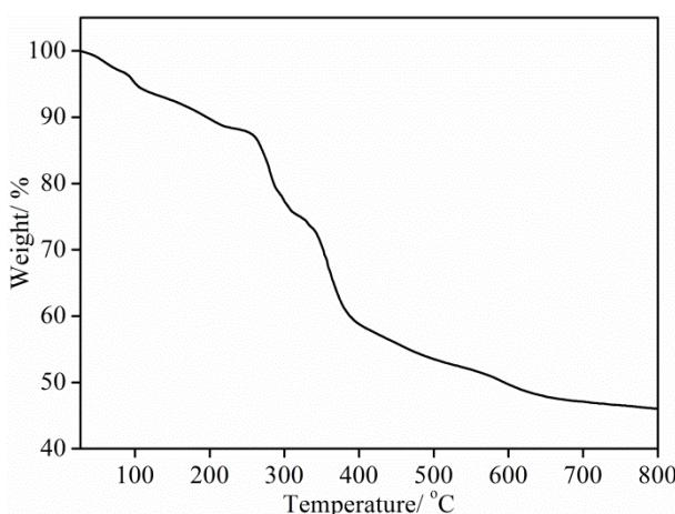
**Figure S24.** TG curve of compound **TOC-12** in  $\text{N}_2$  atmosphere.
