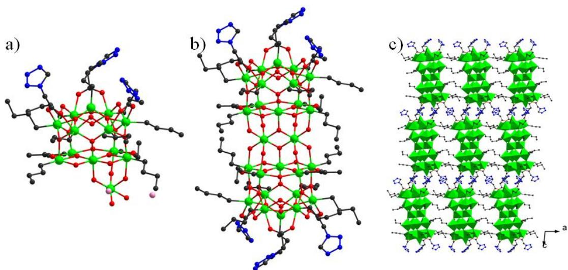
**Figure S5.** The asymmetric unit (a), cluster structure (b), and packing mode (c) of the **TOC-15**. Atom color code: green Sn; red O; black C; dark blue N; pink Cl. Polyhedral color code: green SnO<sub>3</sub>C/SnO<sub>5</sub>C/SnO<sub>6</sub>.
