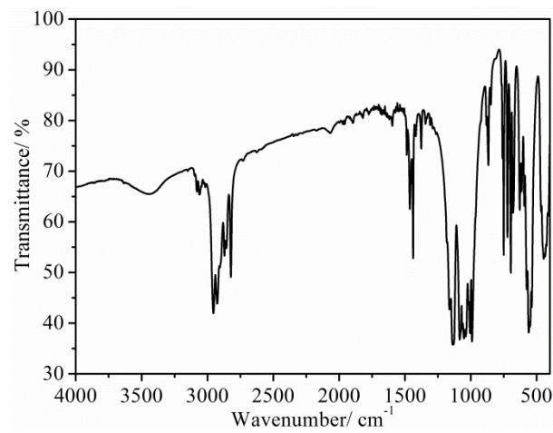
**Figure S18.** IR spectrum of compound **TOC-13**.
