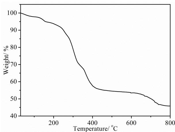
**Figure S28.** TG curve of compound **TOC-16** in N<sub>2</sub> atmosphere.
