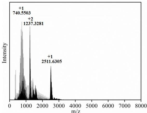
**Figure S41.** The positive-mode ESI-MS spectrum of mother liquor for **TOC-17** diluted by ethanol.
