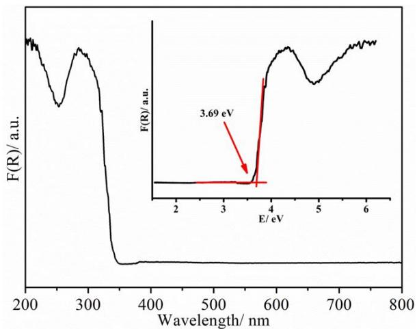
**Figure S34.** UV-vis diffuse reflectance spectrum of **TOC-17**.
