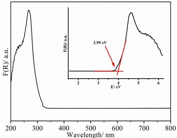
**Figure S35.** UV-vis diffuse reflectance spectrum of **TOC-18**.
