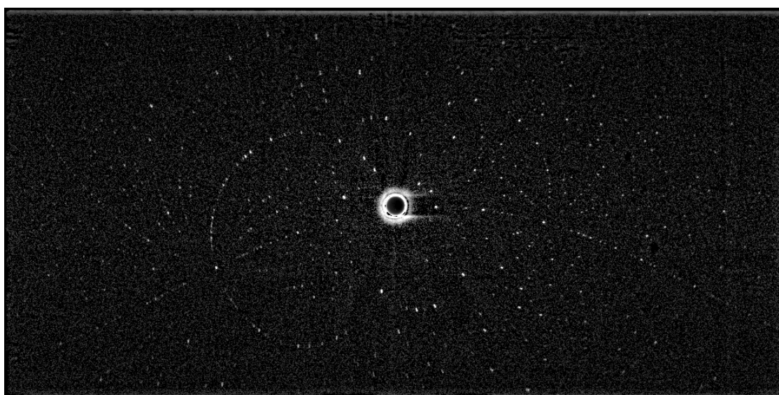
Figure S4.1: A representative Laue image showing the diffraction peaks for which data were extracted for 7c-d 2
