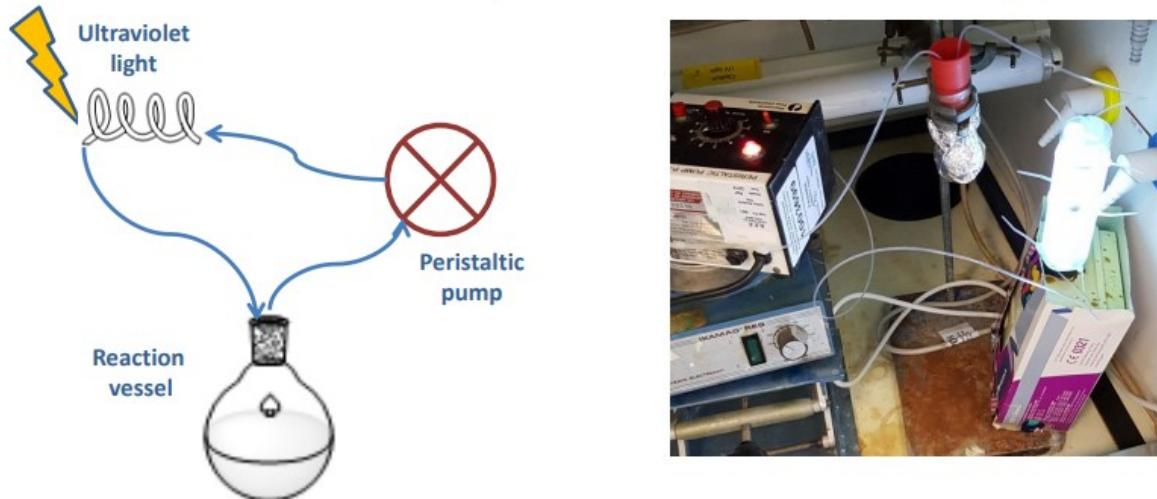
Figure 1: A schematic outlining the flow set-up of the reaction
