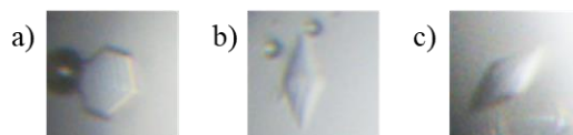
Figure S30. Ice crystal morphology in the presence of synthetic AFGP mimic at 10 mg/mL: a) 15mer AFGP mimic 13c , b) 30mer AFGP mimic 8c , c) 60mer AFGP mimic 9c .
