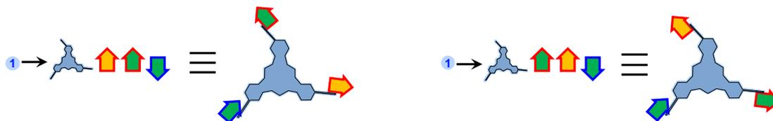
The four possible conformers of the  $S_a, S_a, S_a$  isomer of  $P$ -(TCBD-aniline)<sub>3</sub>-SubPc(<sup>t</sup>BuPhO) **1** resulting from the 180° rotation of each of the three TCBDs around the C-C single bond connecting the SubPc to the tetracyano unit are presented in Figure S3.4.
