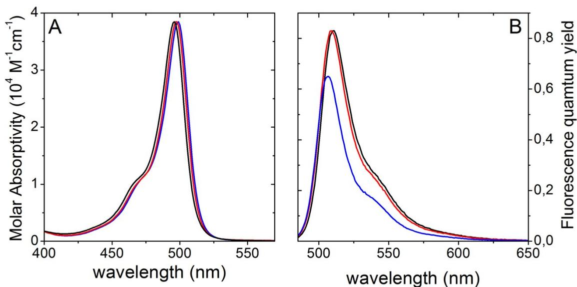
**Figure S2.** Temporal evolution of the absorption and fluorescence spectra of probe (*R*)-BCT-2 dissolved in water: time zero (black), 6 hours (red), and 24 hours (blue).
