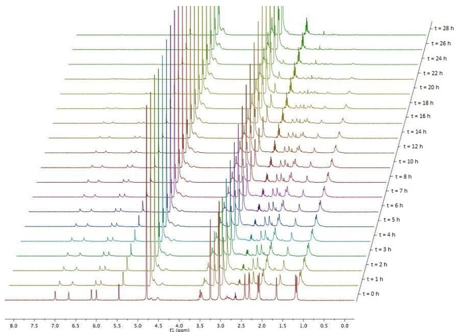
**Figure S1.** NMR study of the stability of the **BCT** probes in  $\text{D}_2\text{O}$  solution.
