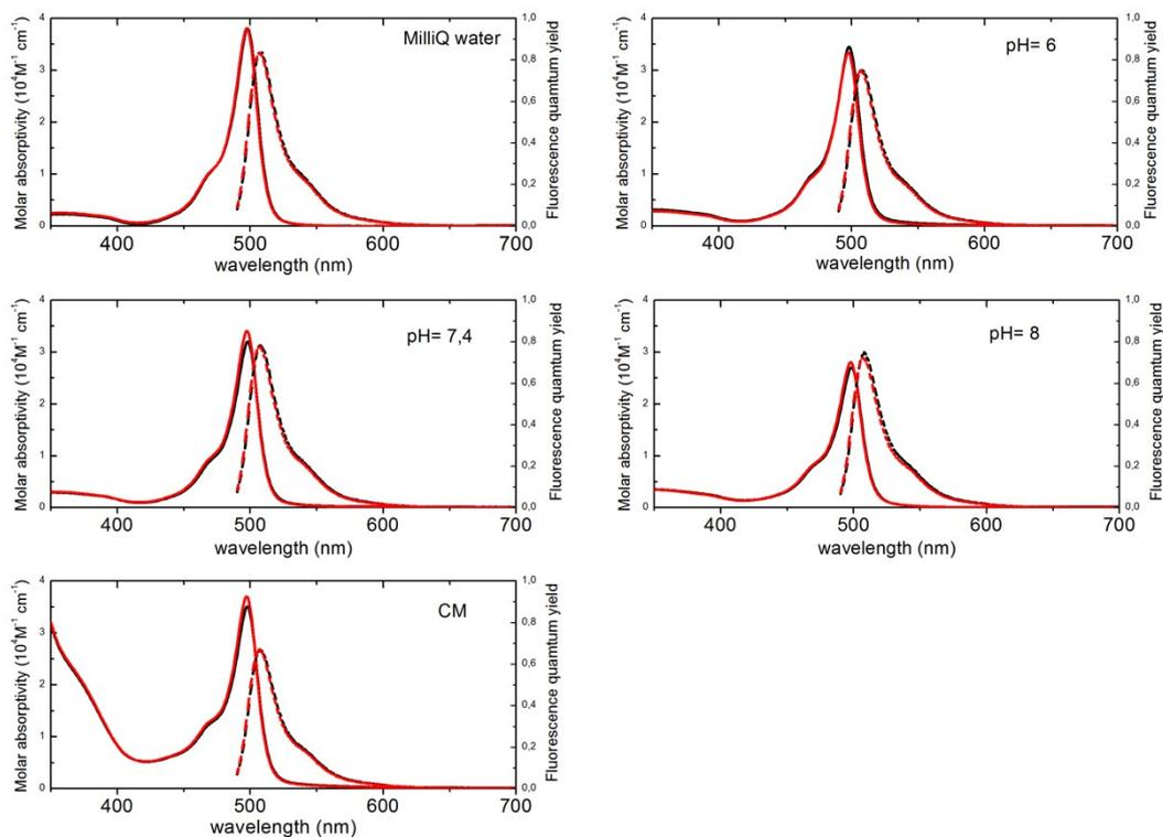
**Figure S3.** Absorption (height-normalized to the molar absorptivity) and emission (height-normalized to fluorescence quantum yield) spectra of (*R*)-**BCT2** in water (for comparison), in PBS (at pH 6.0, 7.4, and 8.0), and in culture medium (CM: Gibco™ DMEM, low glucose, pyruvate, no glutamine, no phenol red culture medium, supplemented with 10% Fetal Bovine Serum, pH 7.4), measured immediately after preparation of the sample (black curves) and after 1h (red curves).
