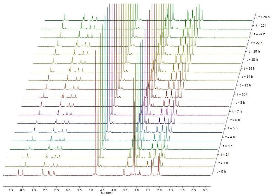
(b) Temporal evolution of the  $^1\text{H}$  NMR spectra of the probe (*R*)-**BCT-2** dissolved in  $\text{D}_2\text{O}$  (15 mM) at 25 °C.
