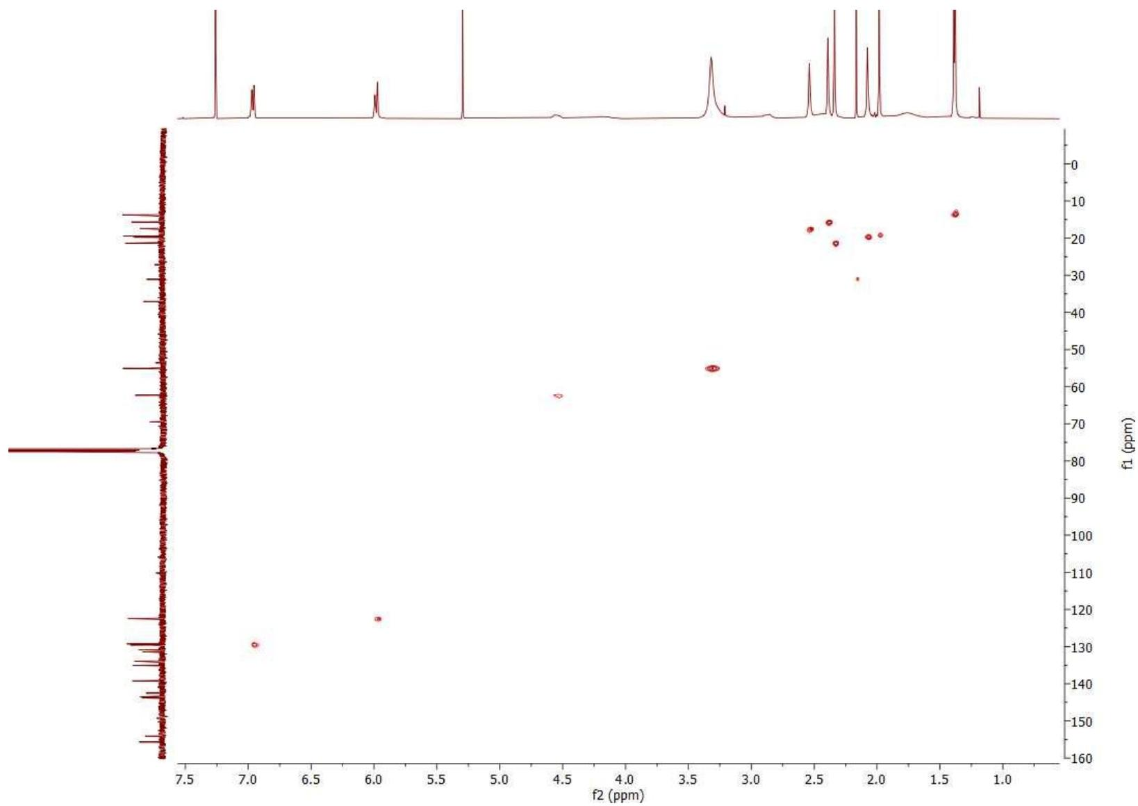
gHSQC (CDCl<sub>3</sub>, 400 MHz) spectrum of (*R*)-**BCT-2**
