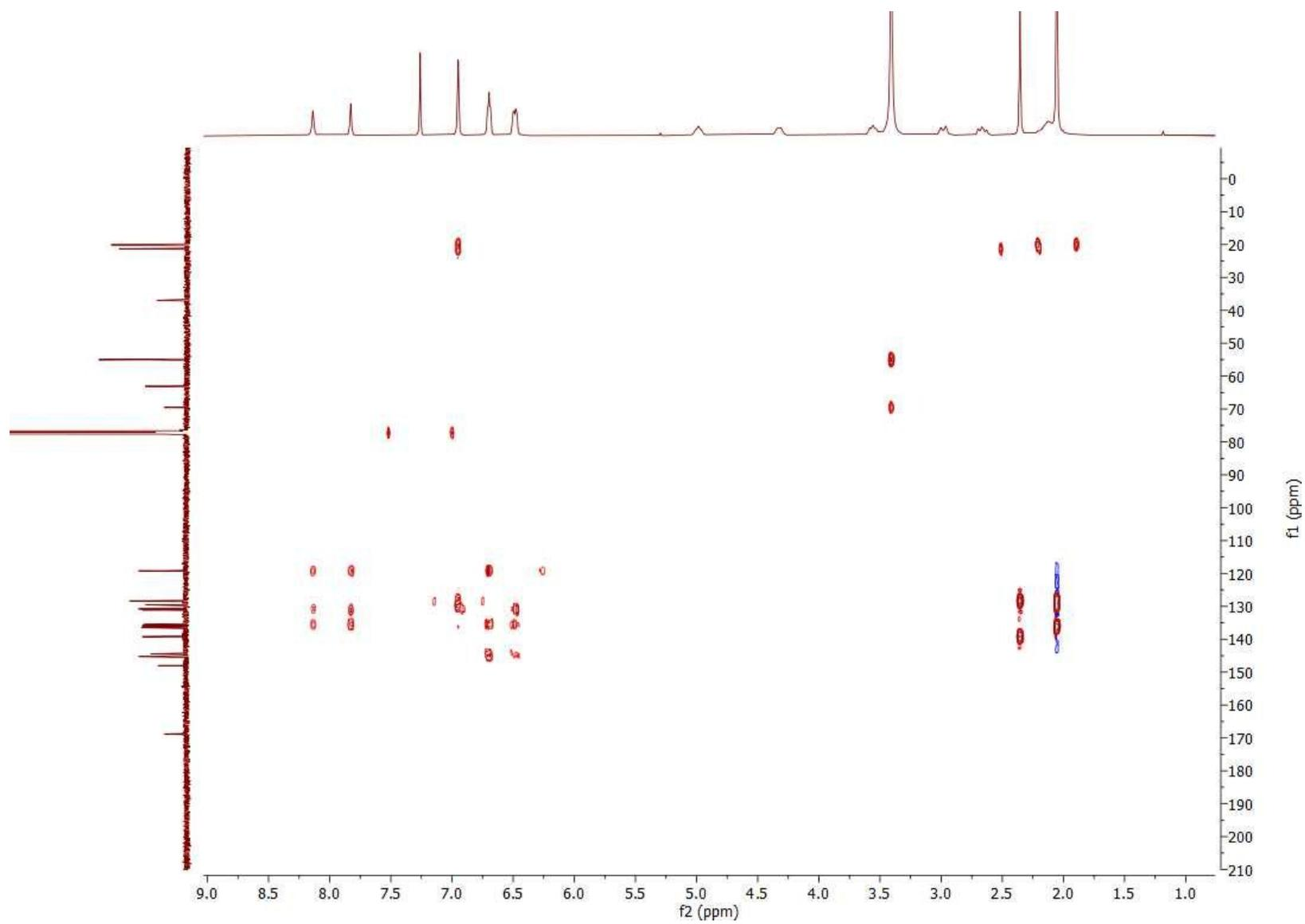
HMBC (CDCl<sub>3</sub>, 400 MHz) spectrum of (*R*)-**BCT-1**
