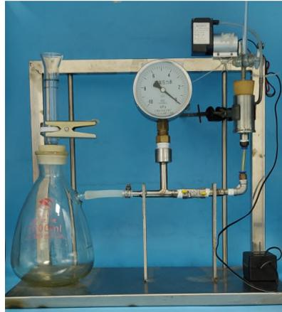
**Fig. S24** Digital image of the home-made vacuum filtration setup.
