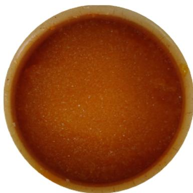
**Fig. S1** Digital image of the PTFE container showing the salt-confined environment during the synthesis of TpPa CONs. In the synthesis system, excessive salt particles were added into the autoclave to create copious confined solid-liquid interfaces. The monomer solution was totally confined in the space among the salt particles.
