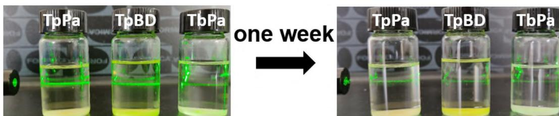
**Fig. S14** Digital images of CONs dispersed in ethanol. After dispersion, the solution showed a strong Tyndall effect, demonstrating the presence of CONs. The prepared CON dispersion maintained stable in ambience for at least one week.
