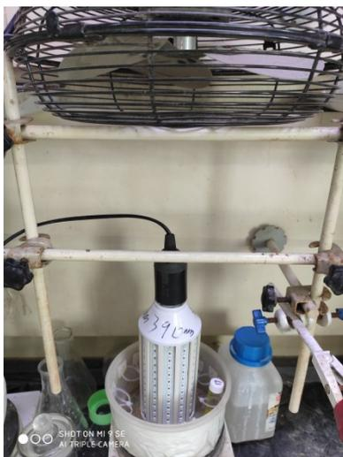
**Figure S1 Photograph of the Photocatalytic reactor used for reactions conducted under 390 nm LED irradiation.**
