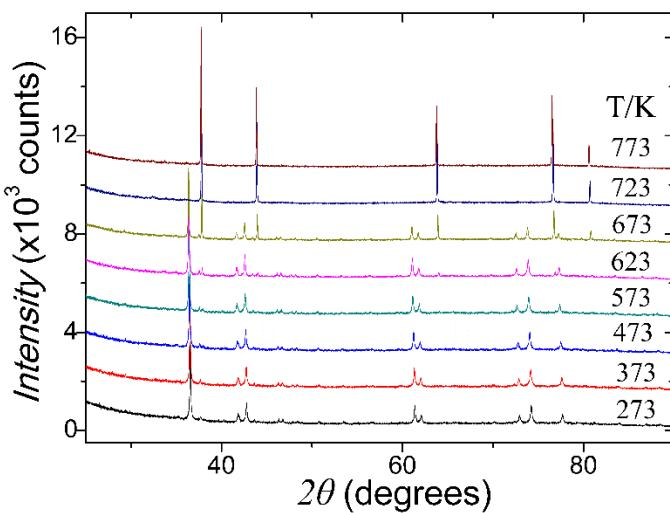
Figure S1. Temperature dependent powder X-ray diffraction indicating  $\text{Ag}_{16}\text{B}_4\text{O}_{10}$  start to decompose into elemental Ag at about 623 K
