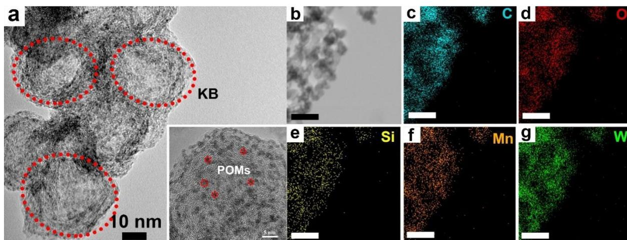
**Figure S27** (a) TEM images of  $\text{SiW}_{12}\text{-MnL}/\text{KB}$  after the catalytic reactions (inset: HR-TEM images of  $\text{SiW}_{12}\text{-MnL}$  after the catalytic). (b–g) Corresponding elemental mapping of C, O, Si, Mn and W of  $\text{SiW}_{12}\text{-MnL}/\text{KB}$  after the catalytic reactions.
