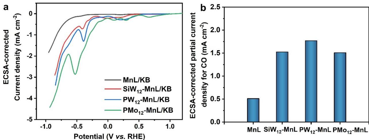
**Figure S23** (a) The ECSA-corrected current density for MnL/KB and POMs-MnL/KB in 0.5 mol L<sup>-1</sup> CO<sub>2</sub>-saturated KHCO<sub>3</sub>, (b) The ECSA-corrected current densities for CO of POM-MnL/KB and MnL/KB.
