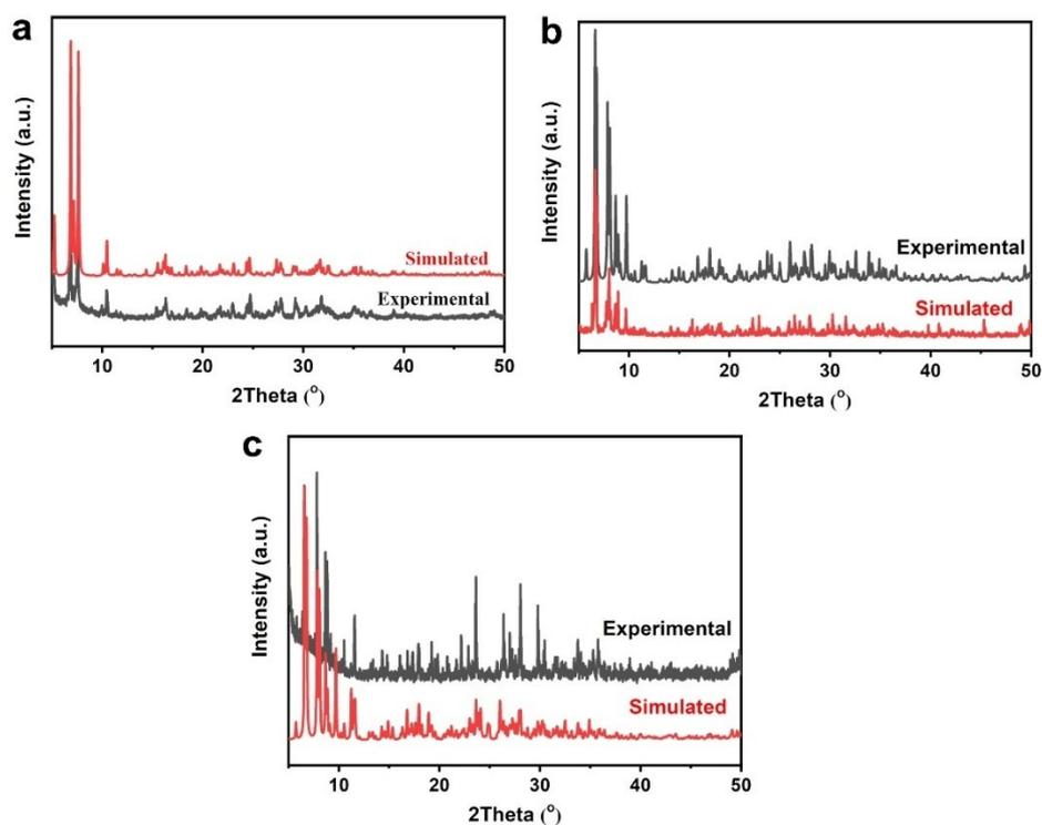
**Figure S4** The powder X-ray diffraction patterns of  $\text{SiW}_{12}\text{-MnL}$  (a),  $\text{PW}_{12}\text{-MnL}$  (b) and  $\text{PMo}_{12}\text{-MnL}$  (c). Powder X-ray diffraction (PXRD, Figure S4) certified the structural integrity and phase purity of the crystalline POM-MnL composite catalysts, the experimental data are consistent with the simulated data are corresponded, which indicates that POM-MnL has been successfully prepared.
