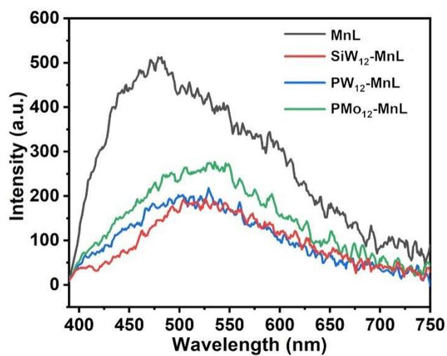
**Figure S29** the fluorescence diagram of MnL and POM-MnL ( $\lambda_{ex}=380$  nm)
