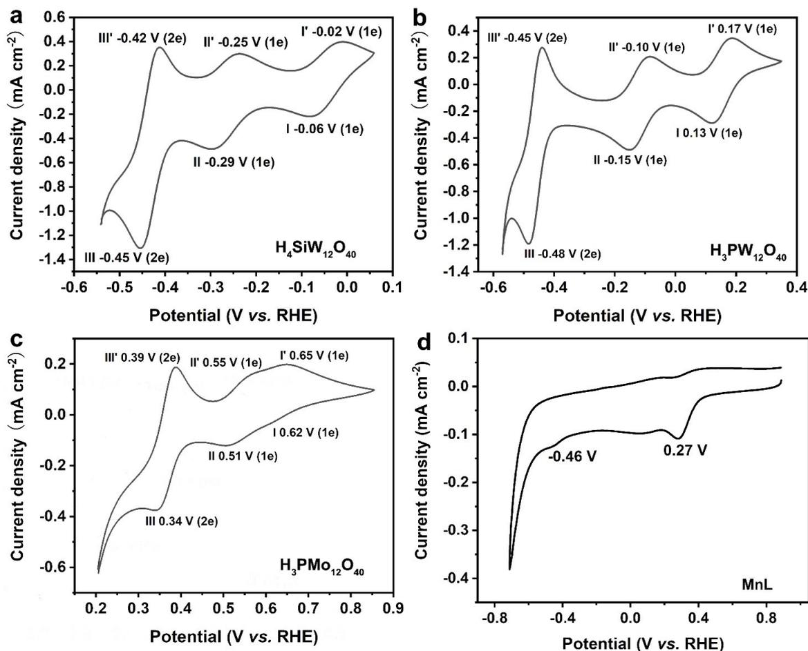
**Figure S15** The CV curves of  $\text{H}_4\text{SiW}_{12}\text{O}_{40}$ (a),  $\text{H}_3\text{PW}_{12}\text{O}_{40}$  (b) ,  $\text{H}_3\text{PMo}_{12}\text{O}_{40}$  (c) in  $0.5 \text{ mol L}^{-1}$   $\text{H}_2\text{SO}_4$  solution (pH 0.3) and MnL in  $0.5 \text{ mol L}^{-1}$   $\text{KHCO}_3$  (pH 8.2) solution at  $0.05 \text{ V s}^{-1}$  scan rate.
