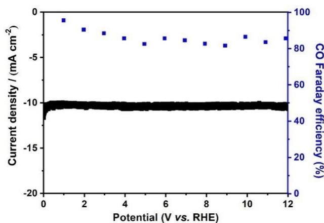
**Figure S26** Changes in current density and FE of  $\text{SiW}_{12}\text{-MnL}$  loaded on KB over 12 h at -0.72 V ( $\eta = 0.61$ ).
