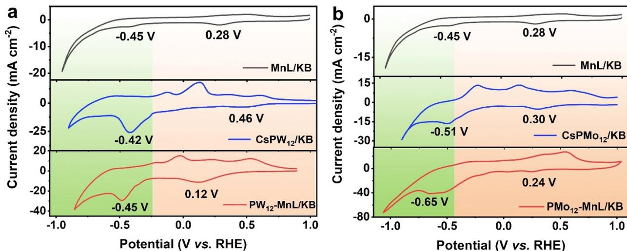
**Figure S16** The CVs for MnL/KB, CsPW<sub>12</sub>/KB and PW<sub>12</sub>-MnL/KB (a) and for MnL/KB, CsPMo<sub>12</sub>/KB and PMo<sub>12</sub>-MnL/KB (b) in 0.5 mol L<sup>-1</sup> N<sub>2</sub>-saturated KHCO<sub>3</sub> at 0.05 V s<sup>-1</sup> scan rate.
