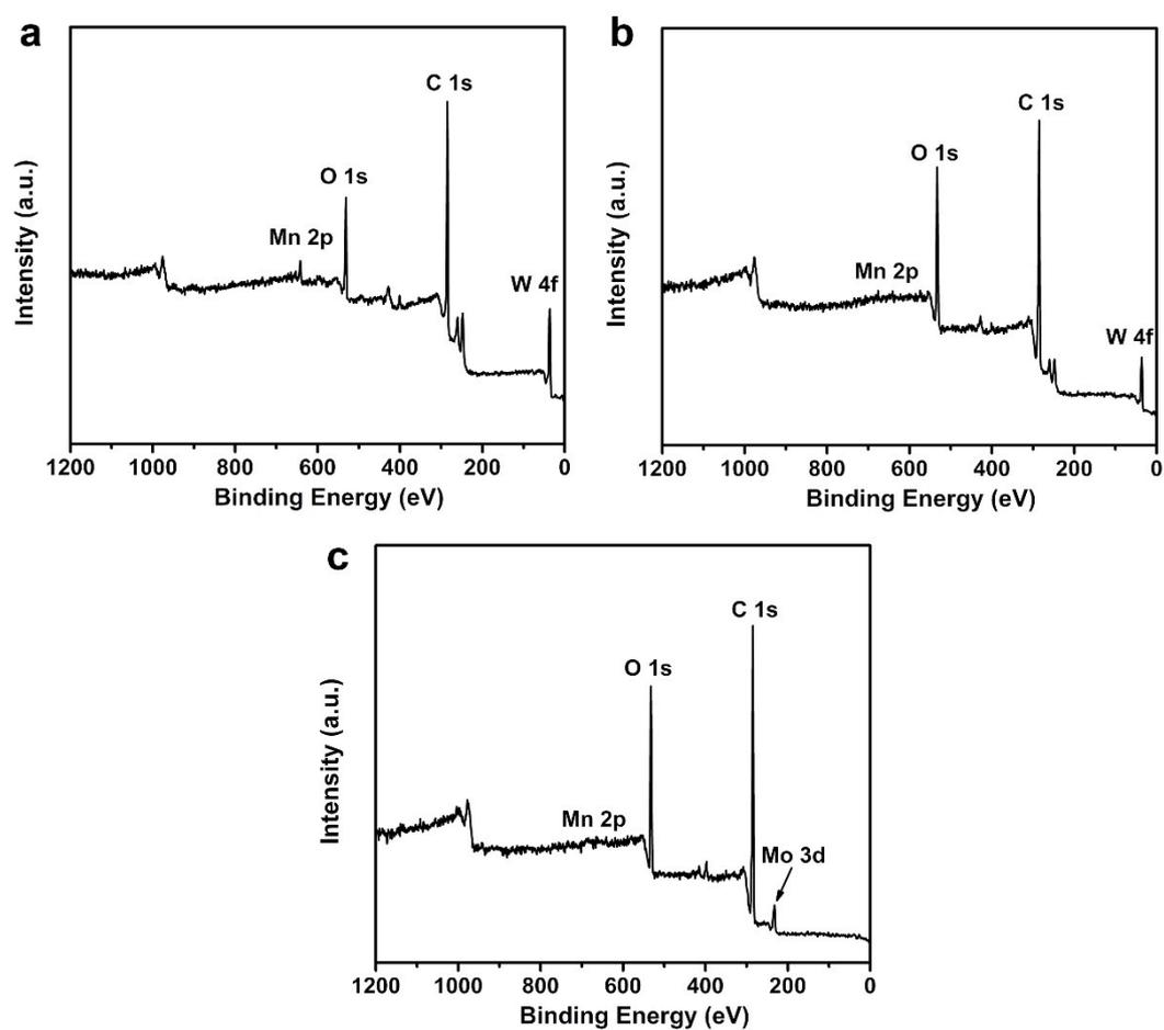
Figure S11 the XPS spectrum of  $\text{SiW}_{12}\text{-MnL/KB}$  (a),  $\text{PW}_{12}\text{-MnL/KB}$  (b) and  $\text{PMo}_{12}\text{-MnL/KB}$  (c).
