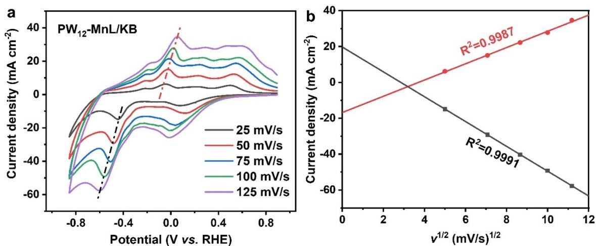
**Figure 18** (a) The CVs for  $\text{PW}_{12}\text{-MnL/KB}$  in  $0.5 \text{ mol L}^{-1} \text{ N}_2\text{-saturated KHCO}_3$  at different scan rate, (b) graph of peak current *vs.* square root of the scan rate.
