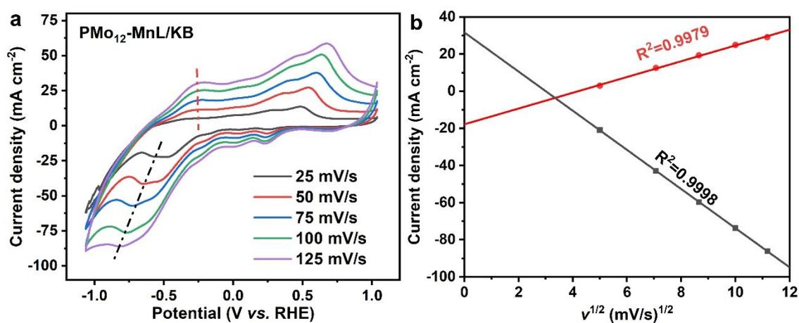
**Figure 19** (a) The CVs for  $\text{PMo}_{12}\text{-MnL/KB}$  in  $0.5 \text{ mol L}^{-1} \text{ N}_2\text{-saturated KHCO}_3$  at different scan rate, (b) graph of peak current *vs.* square root of the scan rate.
