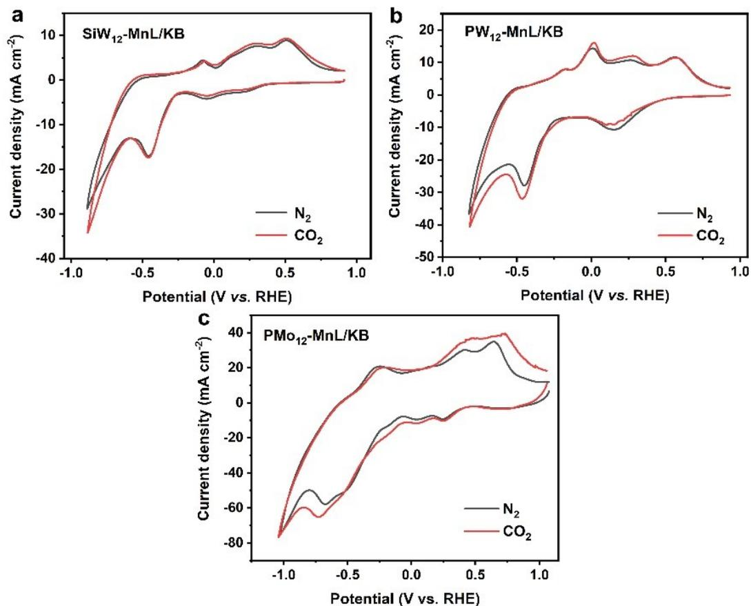
**Figure 20** The CV curves of SiW<sub>12</sub>-MnL/KB (a), PW<sub>12</sub>-MnL/KB (b) and PMo<sub>12</sub>-MnL/KB (c) in 0.5 M N<sub>2</sub>- (black curve) or CO<sub>2</sub>- (red curve) saturated KHCO<sub>3</sub> electrolyte.
