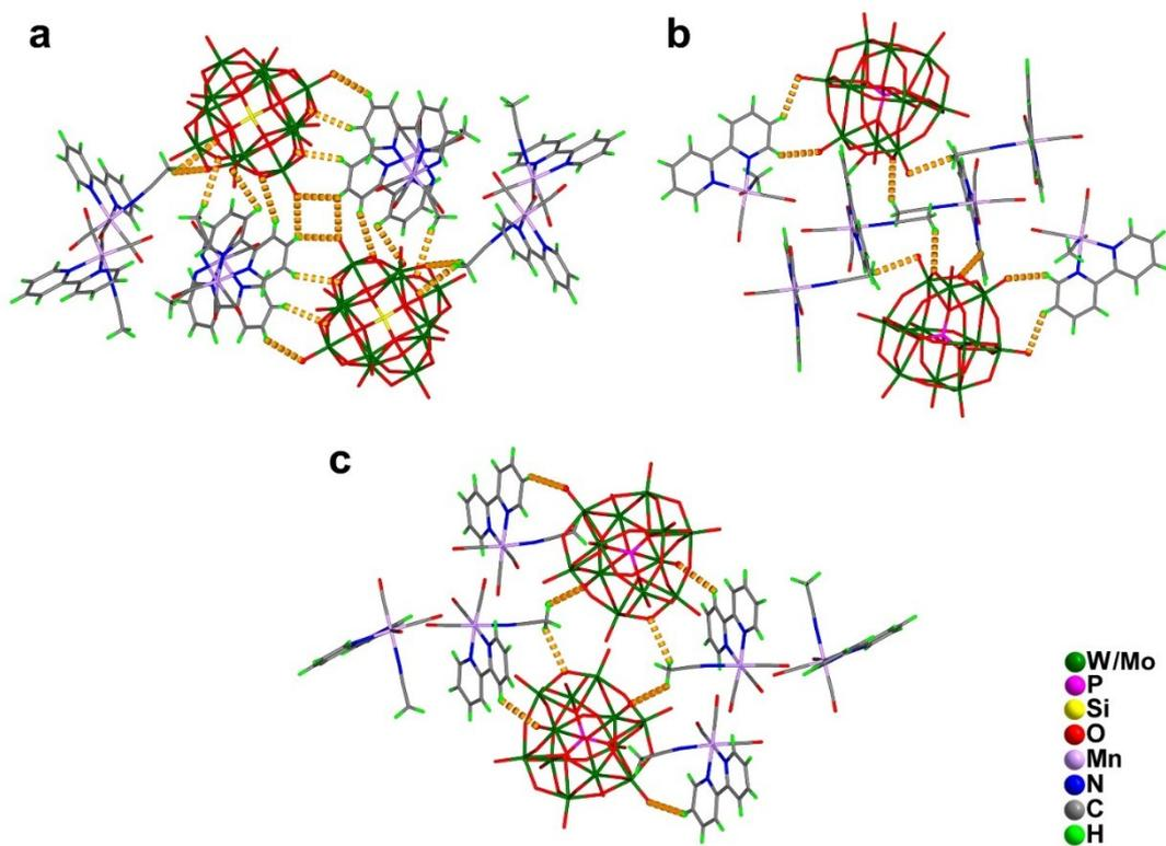
**Figure S3** Hydrogen bonding (orange dotted lines) in the packing arrangement of  $\text{SiW}_{12}\text{-MnL}$  (a)  $\text{PW}_{12}\text{-MnL}$  (b) and  $\text{PMo}_{12}\text{-MnL}$  (c).
