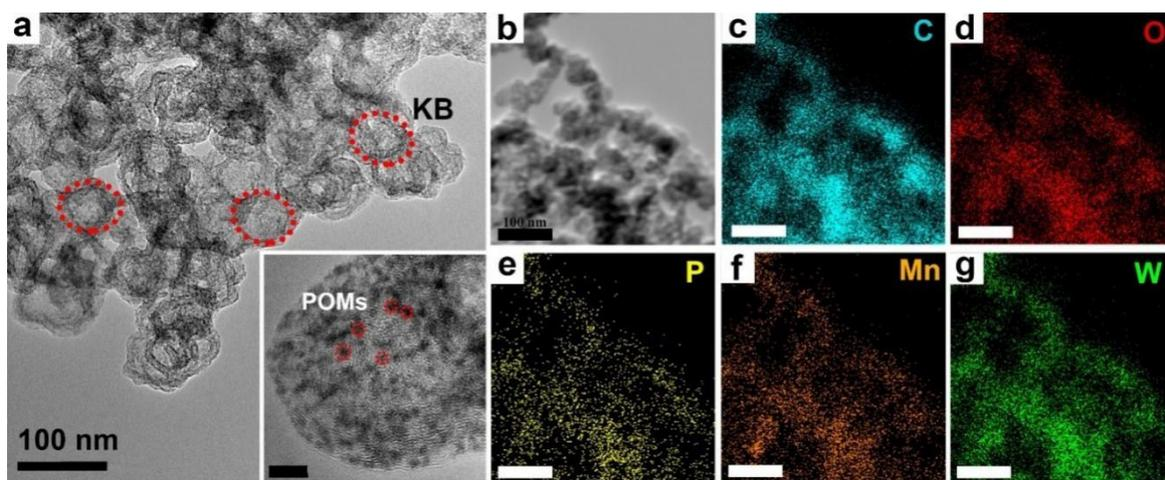
**Figure S8** (a) TEM images of  $\text{PW}_{12}\text{-MnL}$  loaded on KB (inset: HR-TEM images of  $\text{PW}_{12}\text{-MnL}/\text{KB}$ , scale bar: 5 nm). (b–g) Corresponding elemental mapping of C, O, P, Mn and W of  $\text{PW}_{12}\text{-MnL}/\text{KB}$ .
