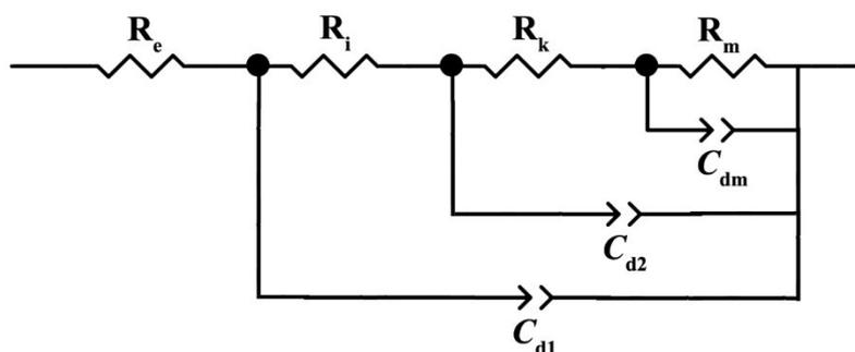
**Figure S25** The equivalent circuit model.
