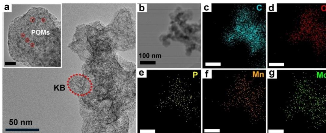
**Figure S9** (a) TEM images of  $\text{PMo}_{12}\text{-MnL}$  loaded on KB (inset: HR-TEM images of  $\text{PMo}_{12}\text{-MnL}/\text{KB}$ , scale bar: 5 nm). (b–g) Corresponding elemental mapping of C, O, P, Mn and Mo of  $\text{PMo}_{12}\text{-MnL}/\text{KB}$ .
