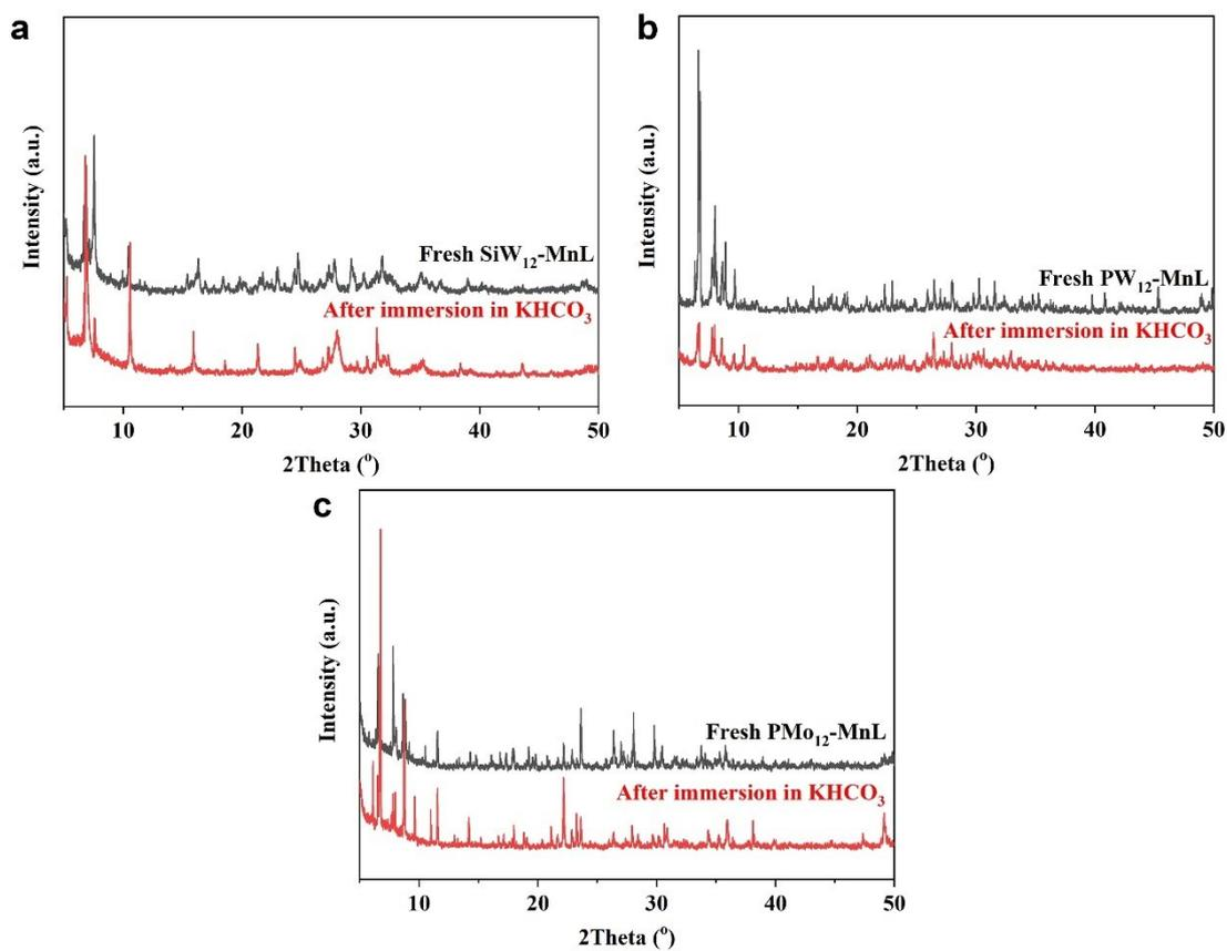
**Figure S7.** XRD patterns of the POMs-MnL after soaking in 0.5 M  $\text{KHCO}_3$  solution.
