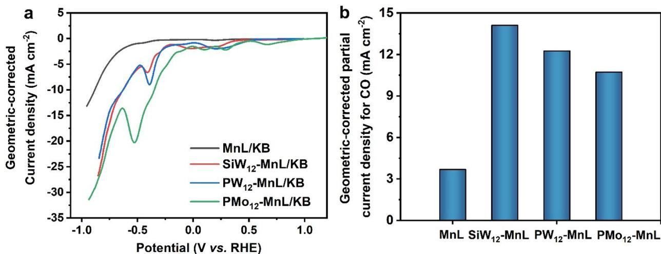
**Figure S21** (a) The geometric-corrected current density for MnL/KB and POMs-MnL/KB in 0.5 mol L<sup>-1</sup> CO<sub>2</sub>-saturated KHCO<sub>3</sub>, (b) The geometric area-corrected current densities for CO of POM-MnL/KB and MnL/KB.
