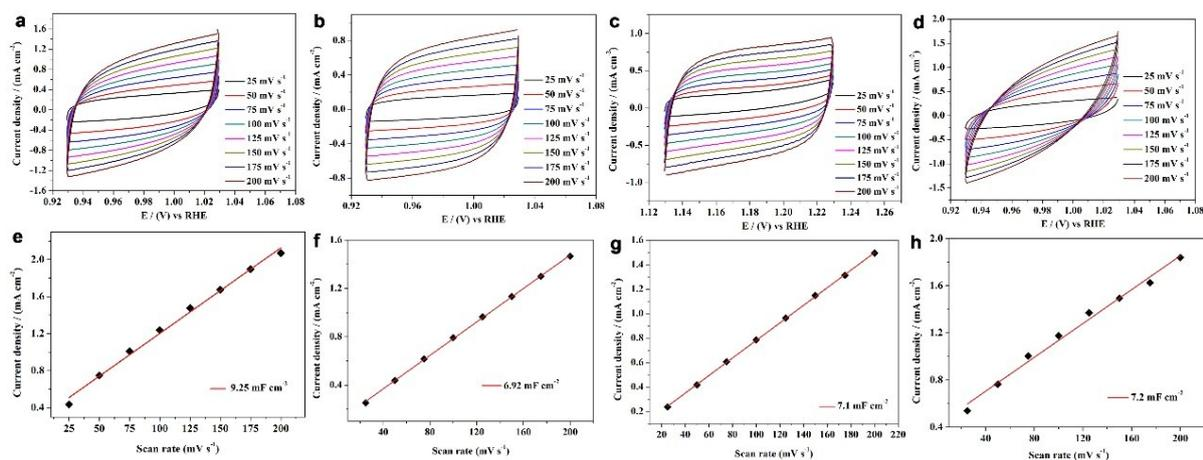
**Figure S22** The CV curve of SiW<sub>12</sub>-MnL/KB (a), PW<sub>12</sub>-MnL/KB (b), PMo<sub>12</sub>-MnL/KB (c) and MnL/KB (d) in the potential range without redox current peaks; the linear fitting of  $\Delta j$  vs. scan rates of SiW<sub>12</sub>-MnL/KB (e), PW<sub>12</sub>-MnL/KB (f), PMo<sub>12</sub>-MnL/KB (g) and MnL/KB (h).
