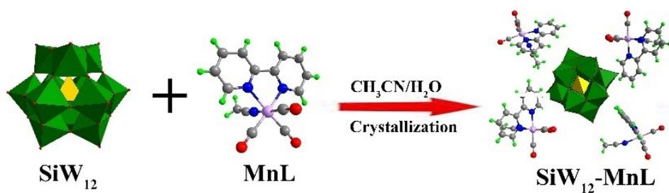
Scheme S1 Illustration of the preparation of  $\text{SiW}_{12}\text{-MnL}$  catalyst.
