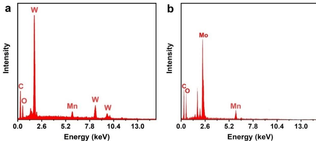
Figure S10 the EDX spectrum of  $\text{PW}_{12}\text{-MnL/KB}$  (a) and  $\text{PMo}_{12}\text{-MnL/KB}$  (b).
