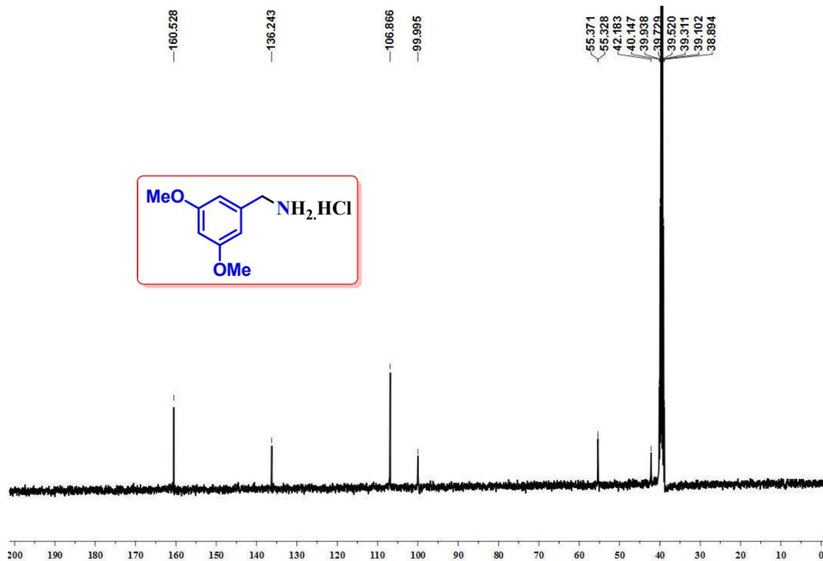
Figure S63. <sup>13</sup>C{<sup>1</sup>H} NMR spectrum of (3,5-dimethoxyphenyl)methanamine hydrochloride (**3x**) in DMSO-d<sub>6</sub>.
