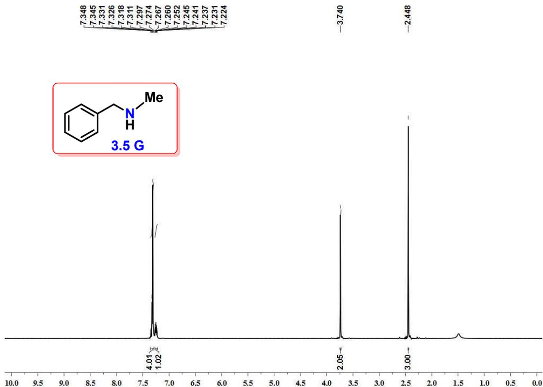
Figure S98.  $^1\text{H}$  NMR spectrum of N-methyl-1-phenylmethanamine (**4'o**) in  $\text{CDCl}_3$ .
