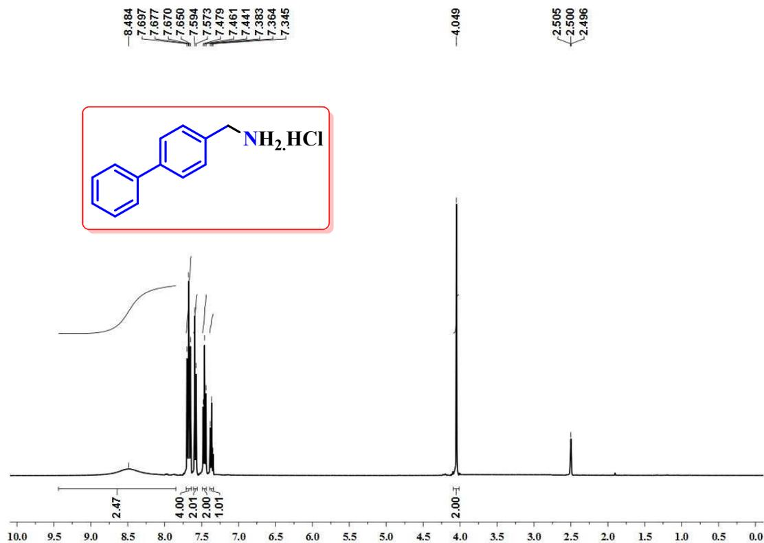
Figure S74. <sup>1</sup>H NMR spectrum of [1,1'-biphenyl]-4-ylmethanamine hydrochloride (**3ae**) in DMSO-d<sub>6</sub>.
