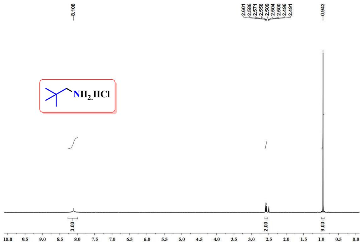
Figure S88. <sup>1</sup>H NMR spectrum of 2,2-dimethylpropan-1-amine hydrochloride (**5j**) in DMSO-d<sub>6</sub>.
