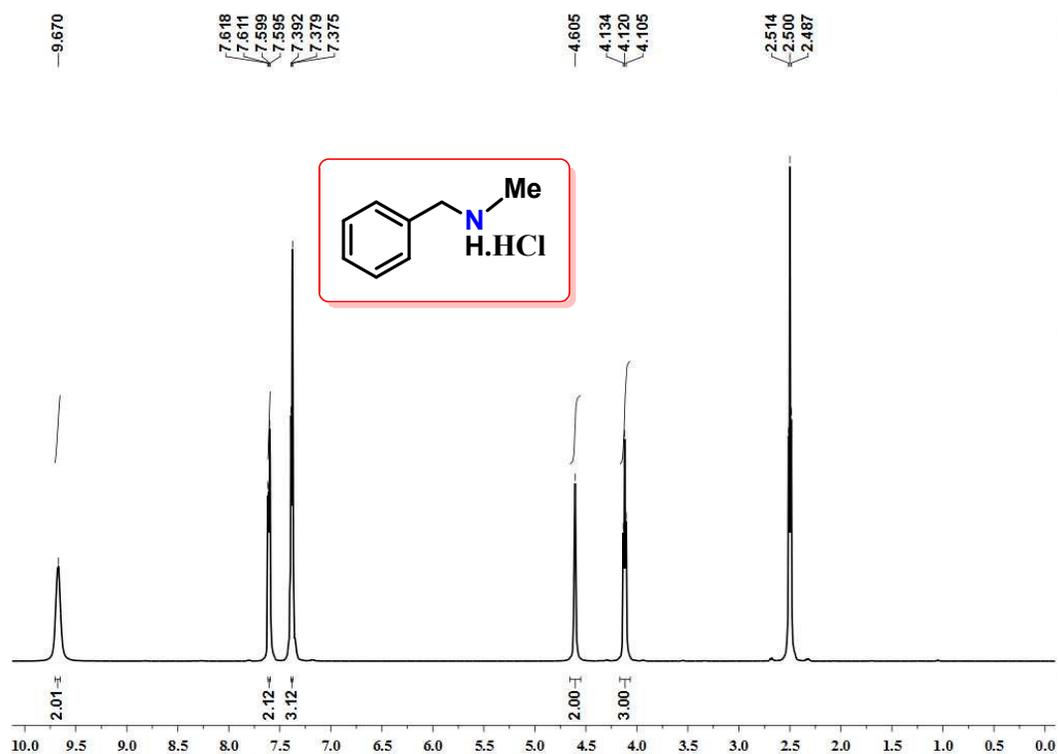
Figure S94.  $^1\text{H}$  NMR spectrum of N-methyl-1-phenylmethanamine hydrochloride (**5n**) in  $\text{DMSO-d}_6$ .
