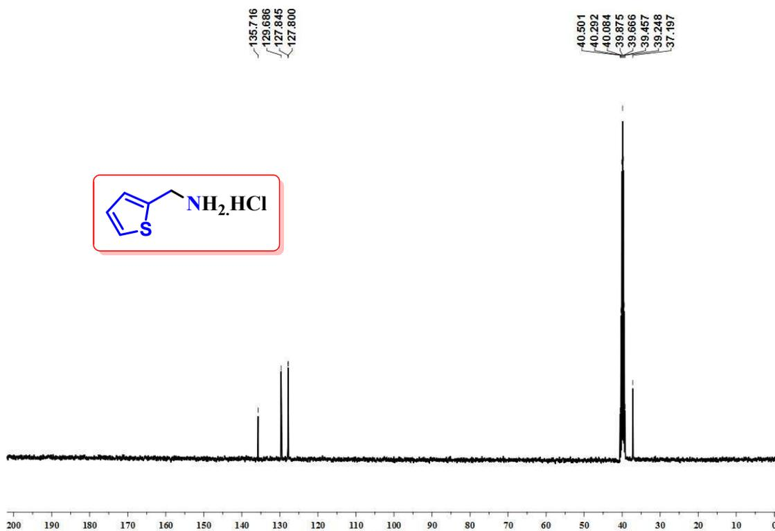
Figure S69. <sup>13</sup>C{<sup>1</sup>H} NMR spectrum of thiophen-2-ylmethanamine hydrochloride (**3aa**) in DMSO-d<sub>6</sub>.
