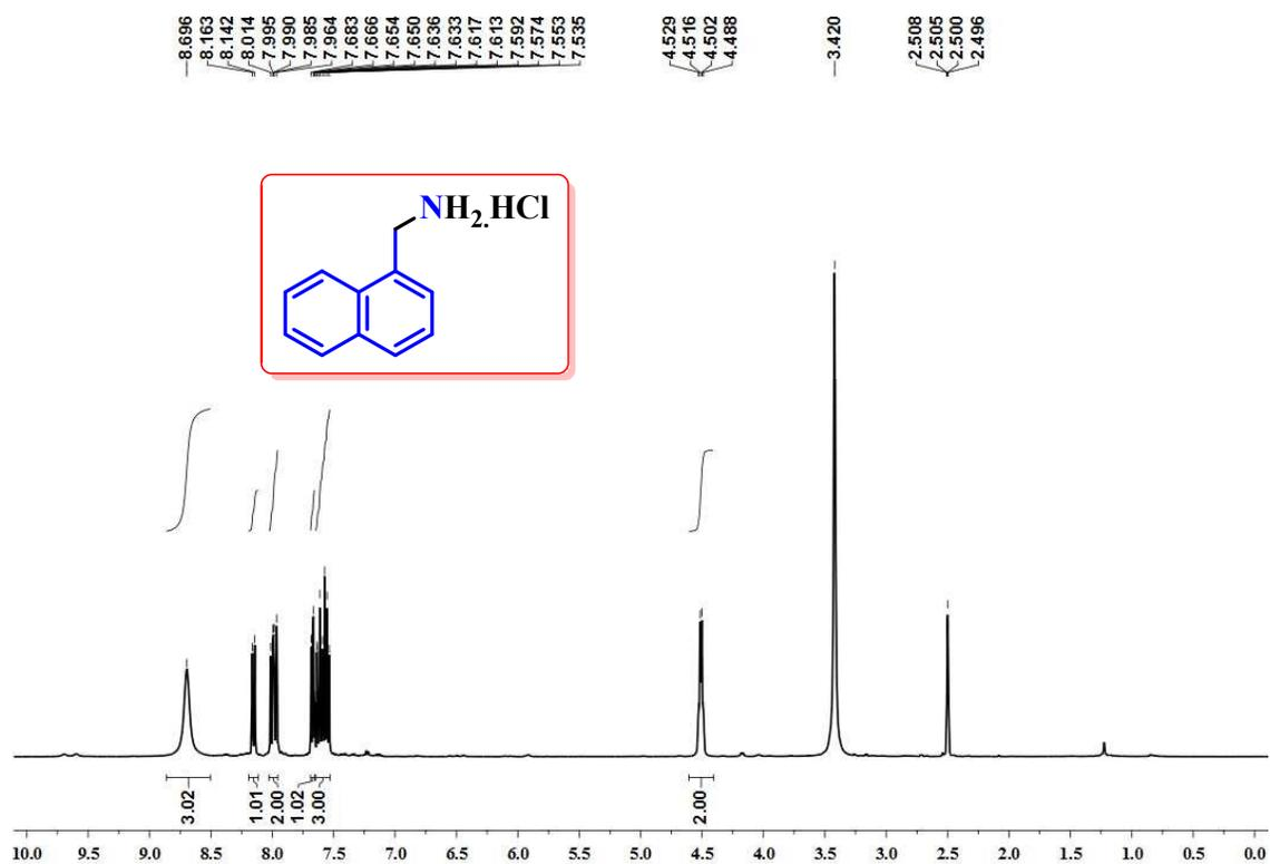
Figure S72. <sup>1</sup>H NMR spectrum of naphthalen-1-ylmethanamine hydrochloride (**3ad**) in DMSO-d<sub>6</sub>.
