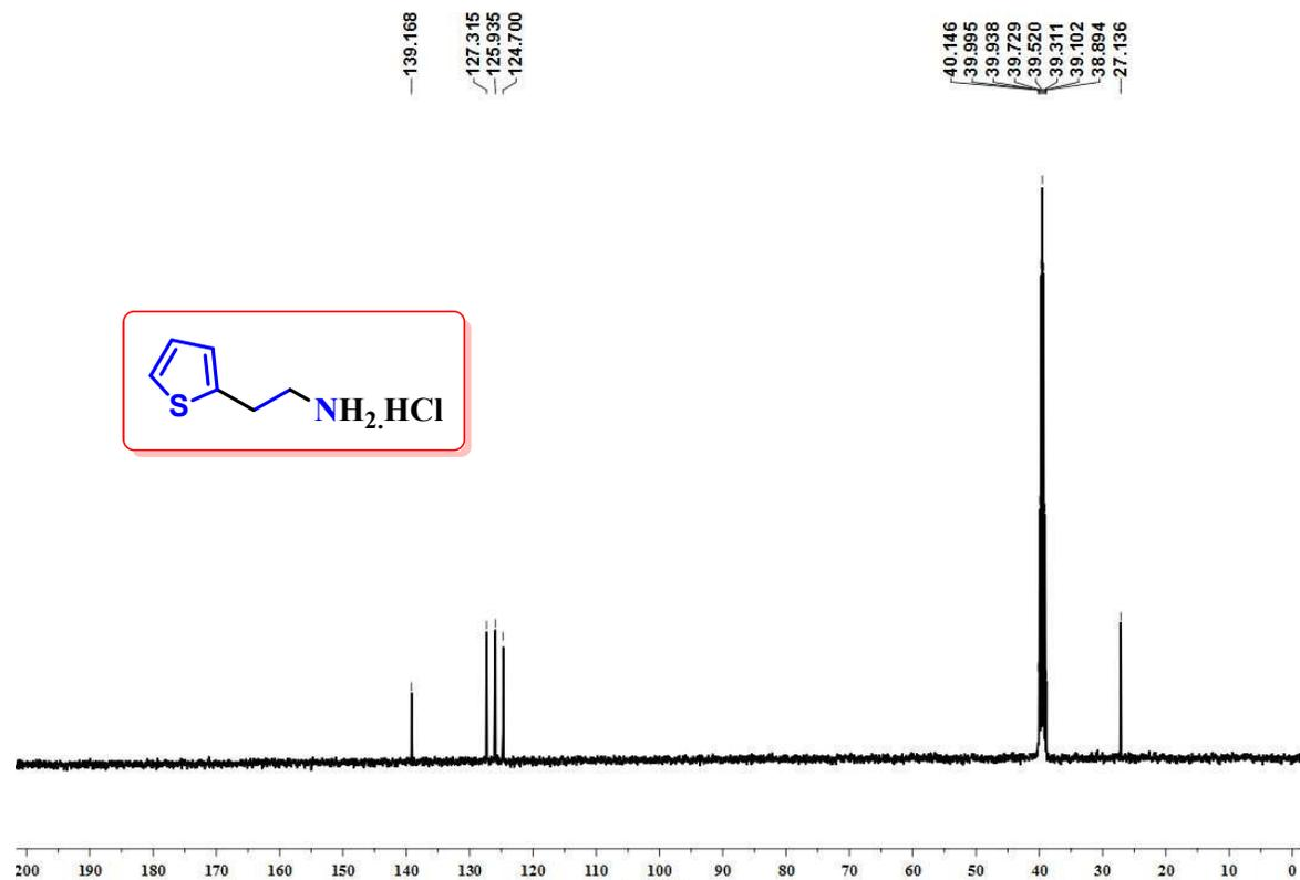
Figure S79.  $^{13}\text{C}\{^1\text{H}\}$  NMR spectrum of 2-(thiophen-2-yl)ethanamine hydrochloride (**5b**) in  $\text{DMSO-d}_6$ .
