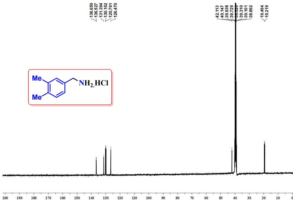
Figure S65. <sup>13</sup>C{<sup>1</sup>H} NMR spectrum of (3,4-dimethylphenyl)methanamine hydrochloride (**3y**) in DMSO-d<sub>6</sub>.
