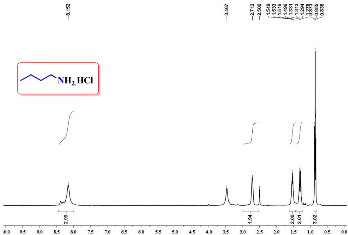
Figure S82.  $^1\text{H}$  NMR spectrum of butan-1-amine hydrochloride (**5g**) in  $\text{DMSO-d}_6$ .
