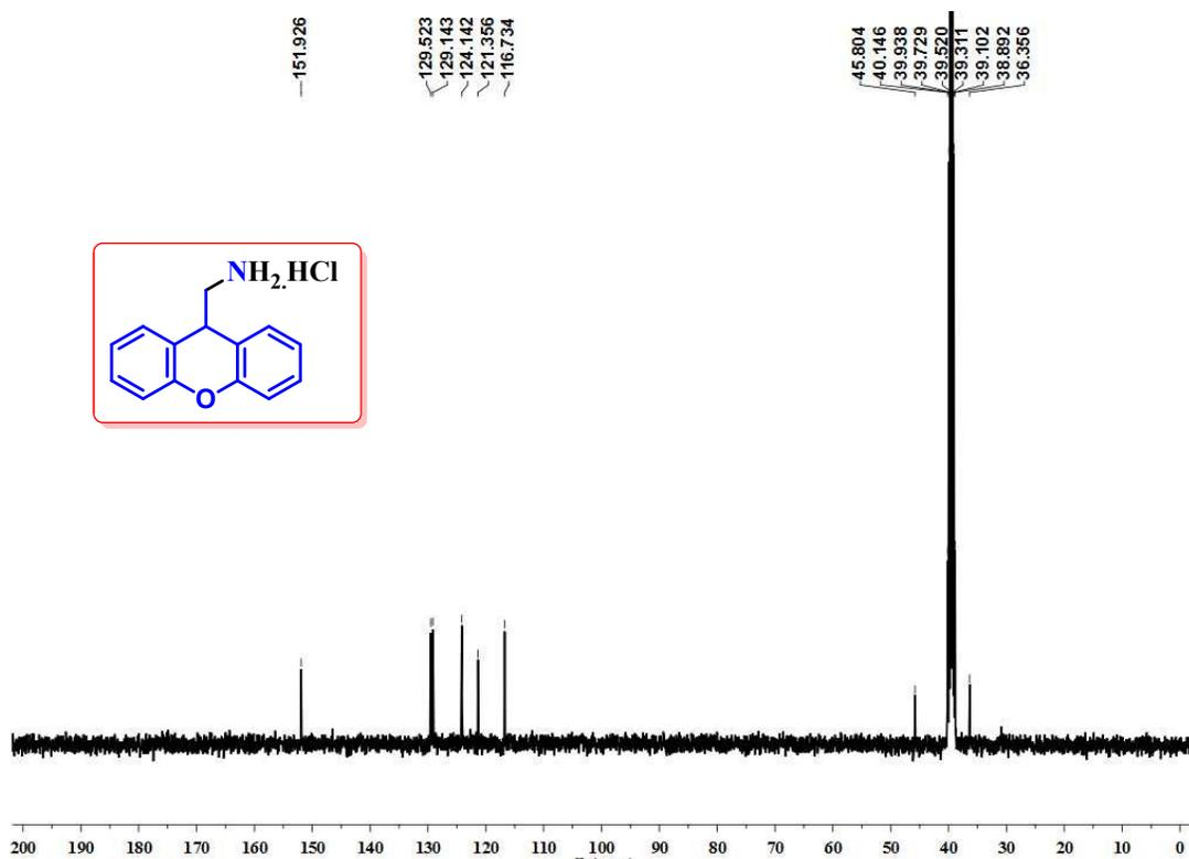
Figure S91. <sup>13</sup>C{<sup>1</sup>H} NMR spectrum of (9H-xanthen-9-yl)methanamine hydrochloride (**5I**) in DMSO-d<sub>6</sub>.
