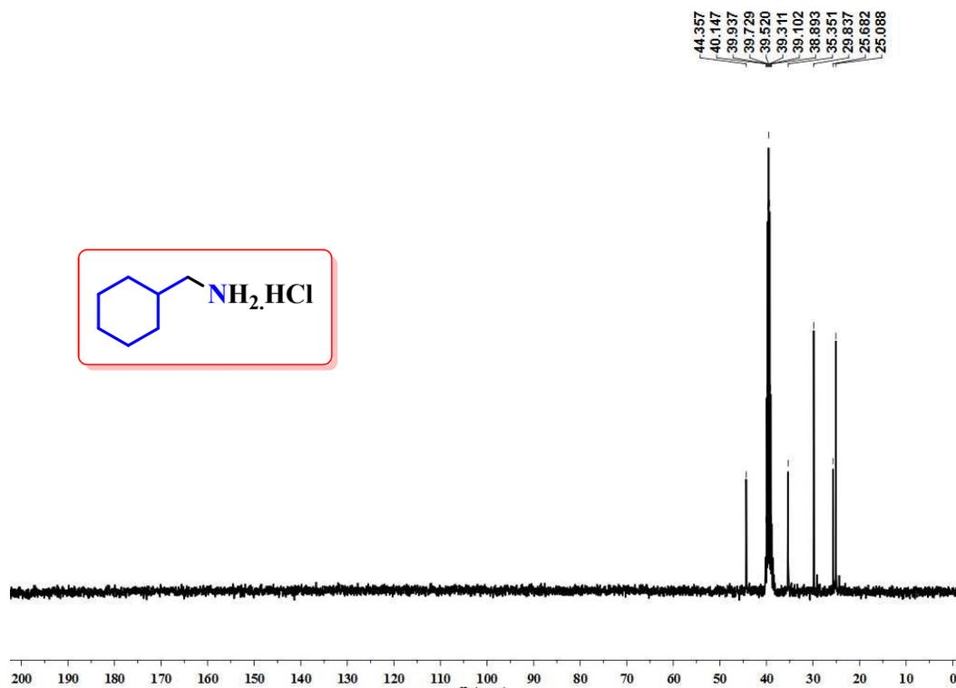
Figure S81.  $^{13}\text{C}\{^1\text{H}\}$  NMR spectrum of cyclohexylmethanamine hydrochloride (**5c**) in  $\text{DMSO-d}_6$ .
