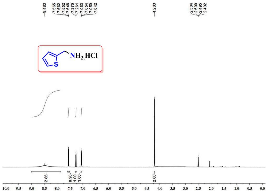
Figure S68. <sup>1</sup>H NMR spectrum of thiophen-2-ylmethanamine hydrochloride (**3aa**) in DMSO-d<sub>6</sub>.
