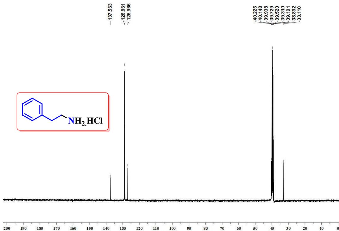
Figure S77. <sup>13</sup>C{<sup>1</sup>H} NMR spectrum of 2-phenylethanamine hydrochloride (**5a**), recorded in DMSO-d<sub>6</sub>.
