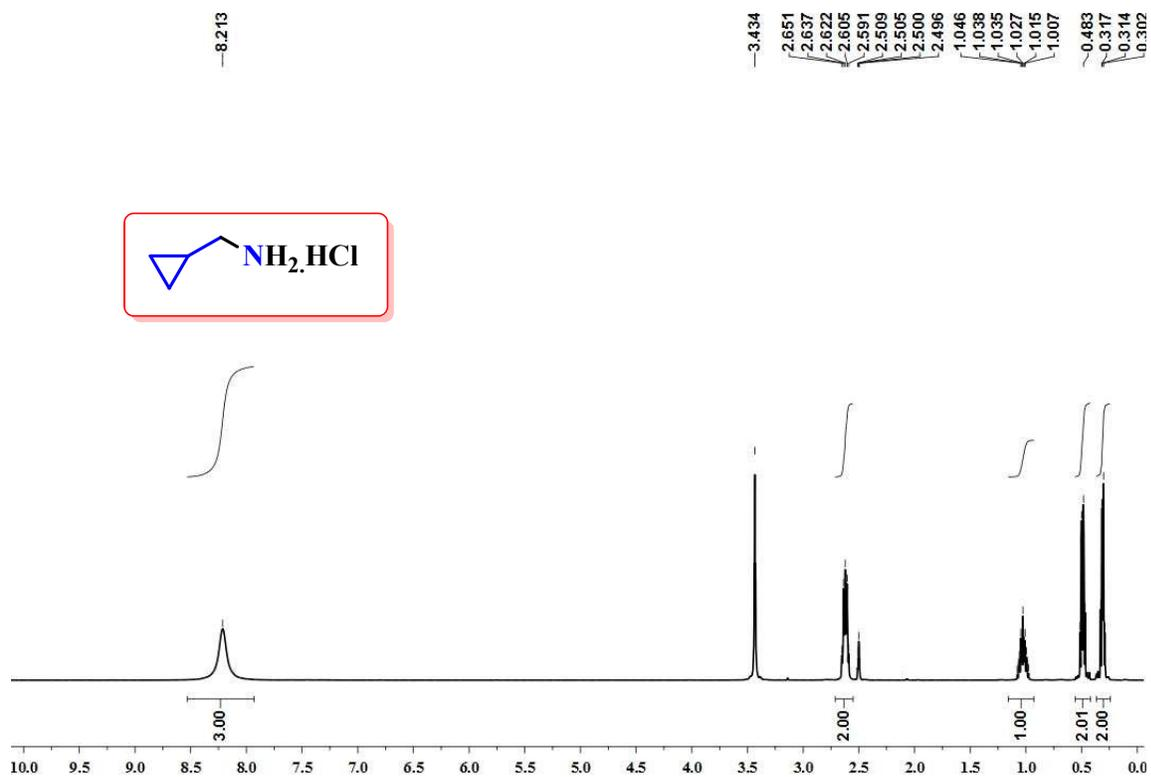
Figure S84.  $^1\text{H}$  NMR spectrum of cyclopropylmethanamine hydrochloride (**5h**) in DMSO- $d_6$ .
