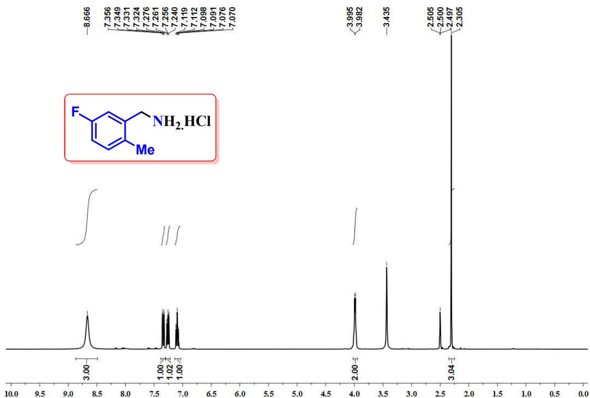
**Figure S60.**  $^1\text{H}$  NMR spectrum of (5-fluoro-2-methylphenyl)methanamine hydrochloride (**3w**) in DMSO- $d_6$ .
