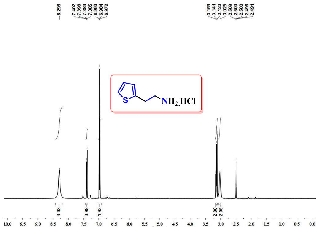
Figure S78.  $^1\text{H}$  NMR spectrum of 2-(thiophen-2-yl)ethanamine hydrochloride (**5b**) in  $\text{DMSO-d}_6$ .
