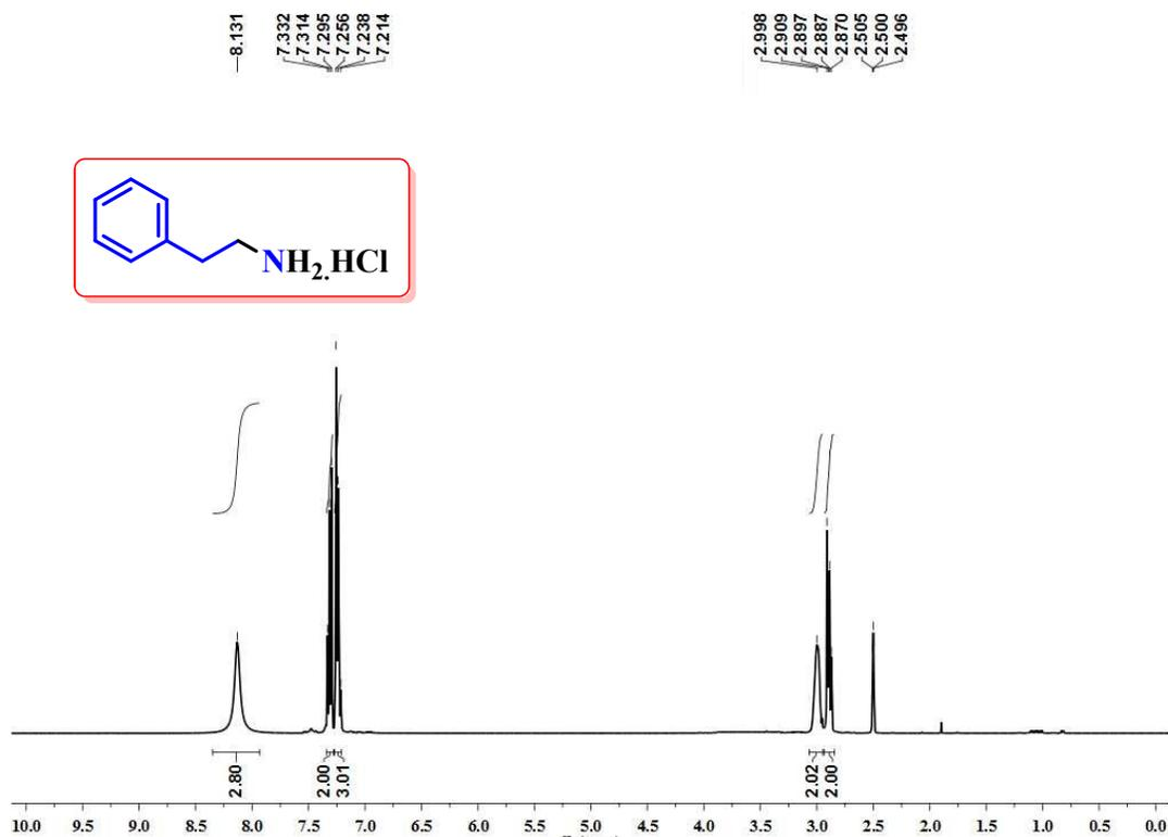
Figure S76. <sup>1</sup>H NMR spectrum of 2-phenylethanamine hydrochloride (**5a**), recorded in DMSO-d<sub>6</sub>.
