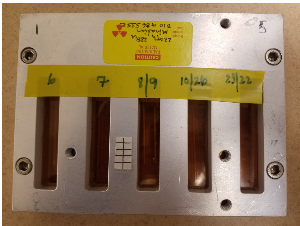
Figure S3: SAXS sample containment. The holder used for radioactive samples is made of aluminum with kapton windows. Inside of the holder, samples in quartz capillaries inside of outer kapton capillaries are taped into slots.
