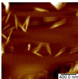
**Figure S6.** The AFM image of the single DNA nanomachine. Phase image: scale bar, 400 nm.
