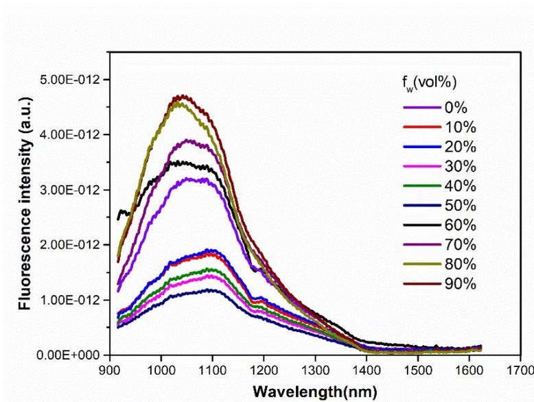
**Figure S4.** Fluorescence emission spectra of **HL2** in water /THF mixtures with different fw (0% to 90%). Excitation wavelength at 785 nm.
