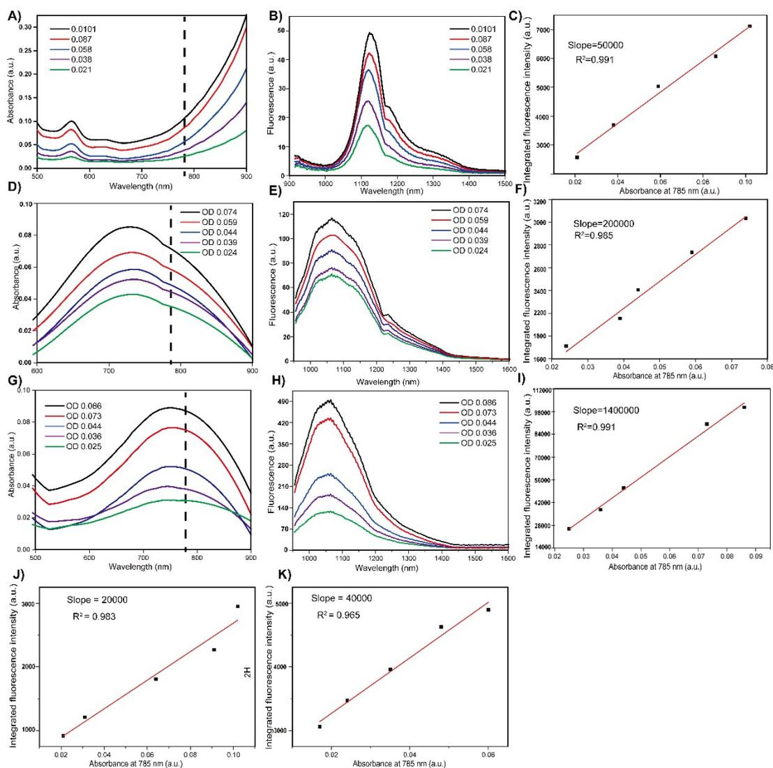
**Figure S3.** Fluorescence quantum yield measurements of **HL3** in THF. The method was reported in our previous work <sup>[1]</sup> and IR-26 is the reference with 0.5% quantum yield in DCE. Absorbance (A, D, G) and fluorescence (B, E, H) spectra of IR-26 in
