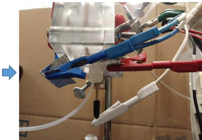
Figure S5. Steps in cell construction, from laying down the Pt electrode to connecting the closed cell to potentiostat cables.
