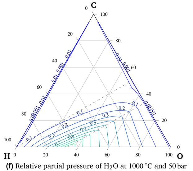
**Figure S1** Relative partial pressures of H<sub>2</sub>O.
