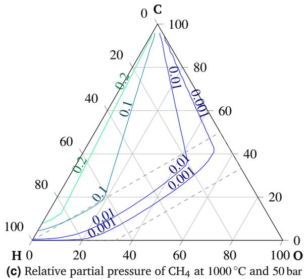
**Figure S2** Relative partial pressures of CH<sub>4</sub> at 50 bar
