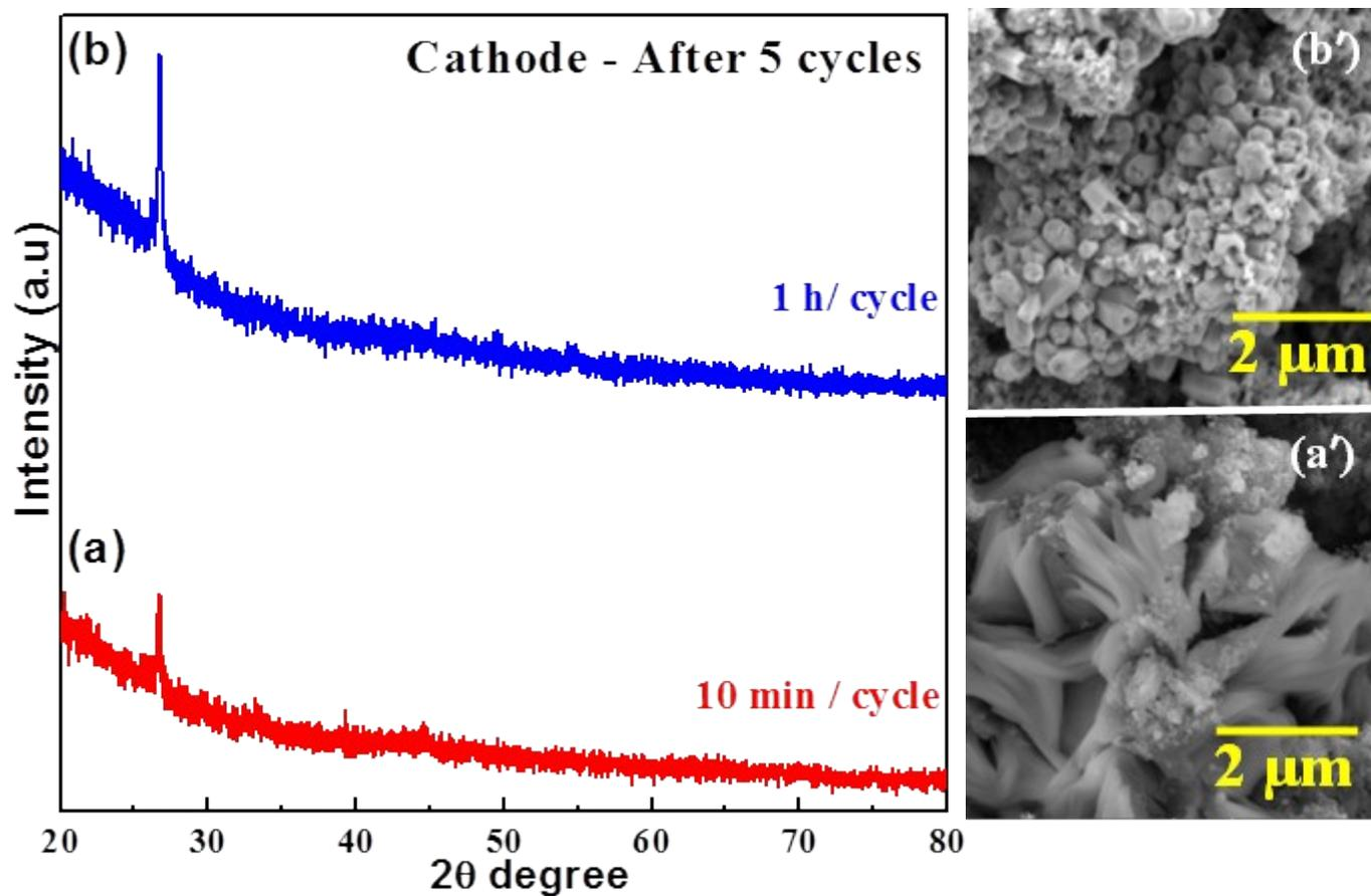
*Fig. S7 XRD pattern and FE-SEM images of cathode at different time duration: 10 minutes / cycle (a,a') and 1 hour / cycle (b,b') respectively*
