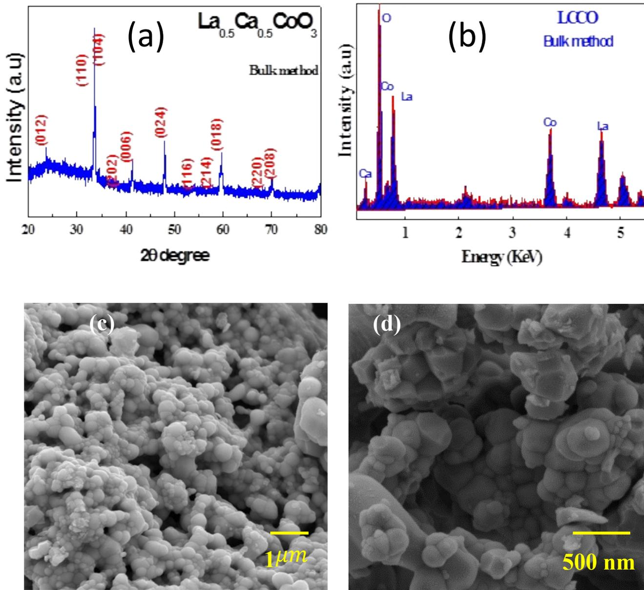
*Fig. S1 (a) XRD pattern, (b) EDX profile (c-d) FE-SEM images of bulk LCCO*
