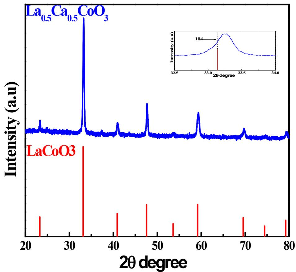
*Fig. S3 Comparison of  $\text{La}_{0.5}\text{Ca}_{0.5}\text{CoO}_3$  X-ray diffraction pattern with parent  $\text{LaCoO}_3$*
