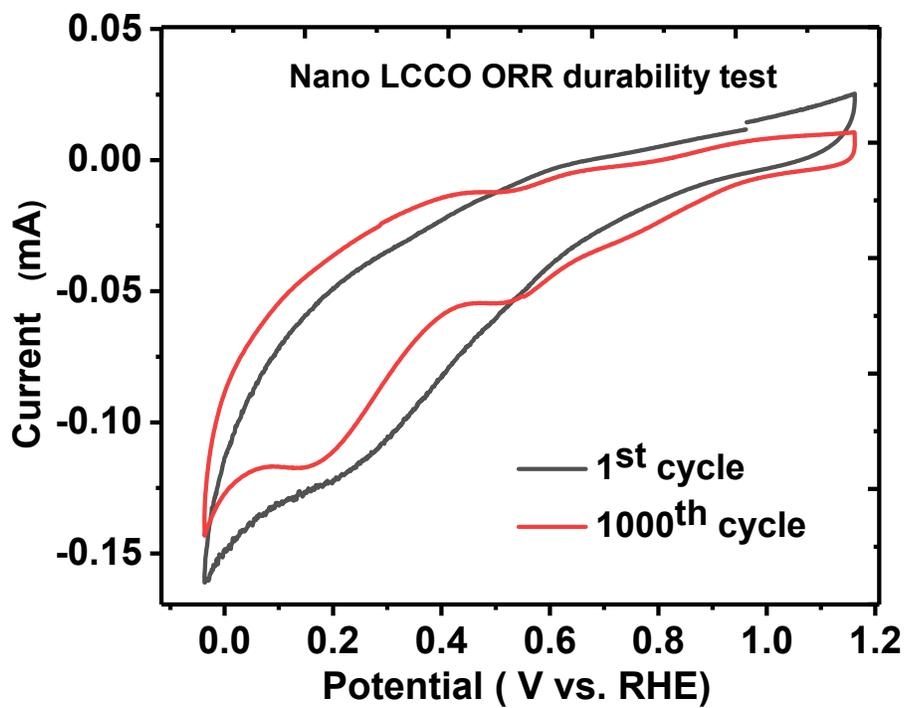
*Fig. S5 CV curves over time of stability testing (0.0–1.2 V vs. RHE, O<sub>2</sub>-saturated 0.1 M KOH solution) for nano LCCO*
