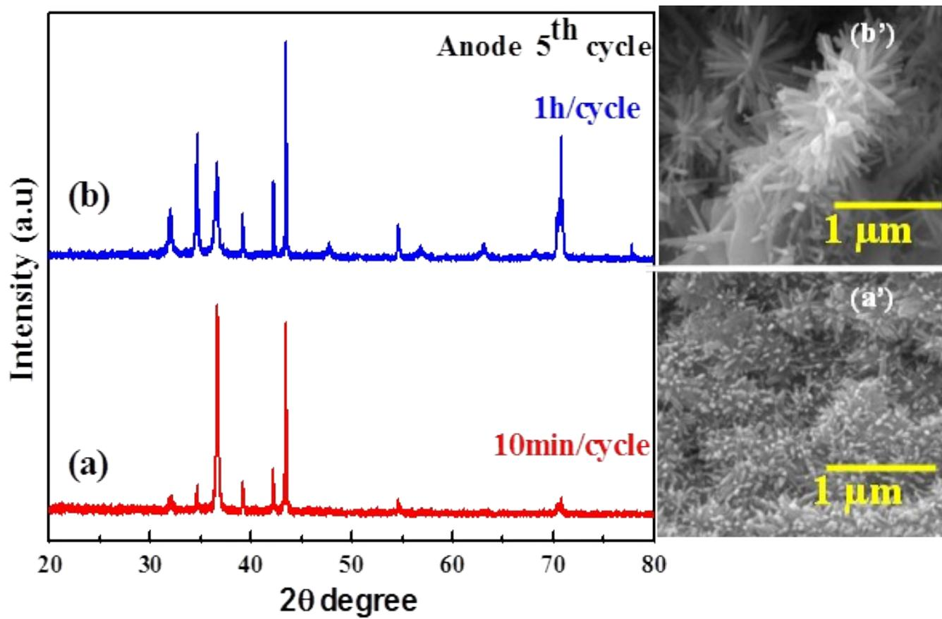
**Fig.S8** XRD pattern and FESEM images of anode at different time duration:(i) 10 minutes / cycle (a,a') and 1 hour / cycle (b,b') respectively
