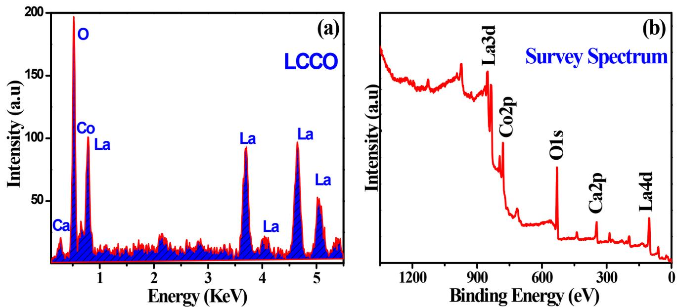
*Fig. S2 (a) EDX profile and (b) XPS survey spectrum of the nano LCCO*
