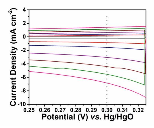
Fig. S2 CV curves of  $Ni_2P_2O_7$  electrode at different scan rates on a potential range of 0.250 to 0.325 V vs. Hg/HgO.
