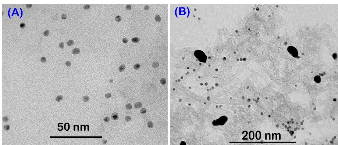
**Figure S8.** The TEM of Au@HP5 (A) and Au@SWCNT (B), respectively.
