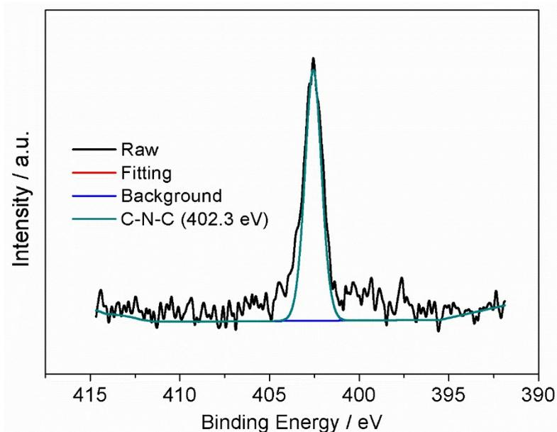
**Figure S9.** High resolution XPS spectra of N 1s for Au@HP5@SWCNT.
