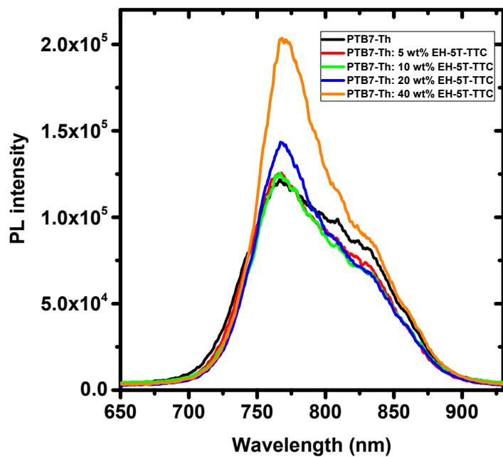
**Figure 10.** Photoluminescence spectra of **PTB7-Th** and blends of **PTB7-Th:EH-5T-TTC**.
