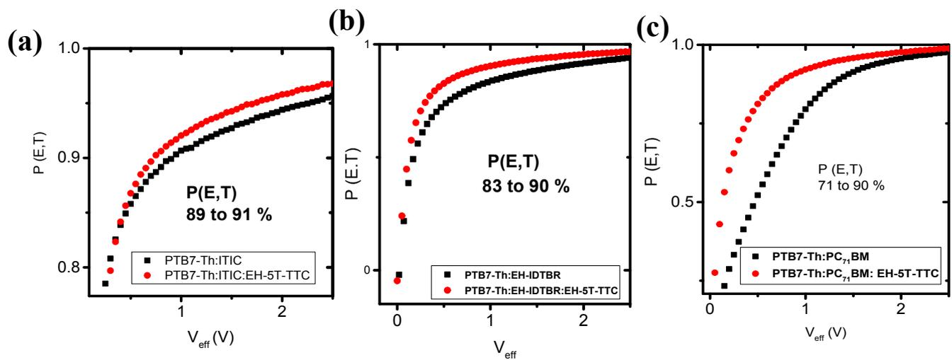
**Figure S9.** Comparison of the exciton dissociation probability of binary and ternary blends of (a) PTB7:ITIC (b) PTB7-Th:EH-IDTBR and (c), PTB7-Th:PC<sub>71</sub>BM with EH-5T-TTC
