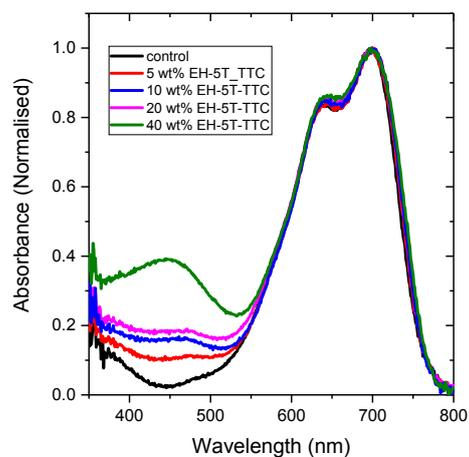
**Figure S3.** UV-Vis absorption spectra of the **PTB7-Th:ITIC** as a function of different **EH-5T-TTC** content.
