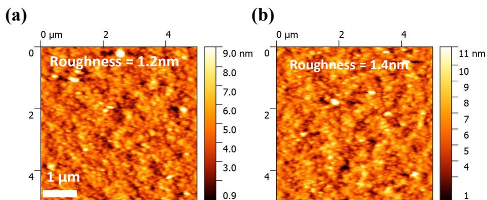
**Figure S7.** Atomic force microscopy images of the (a) **PTB7-Th:ITIC** and (b) **PTB7-Th:ITIC:EH-5T-TTC** blend films
