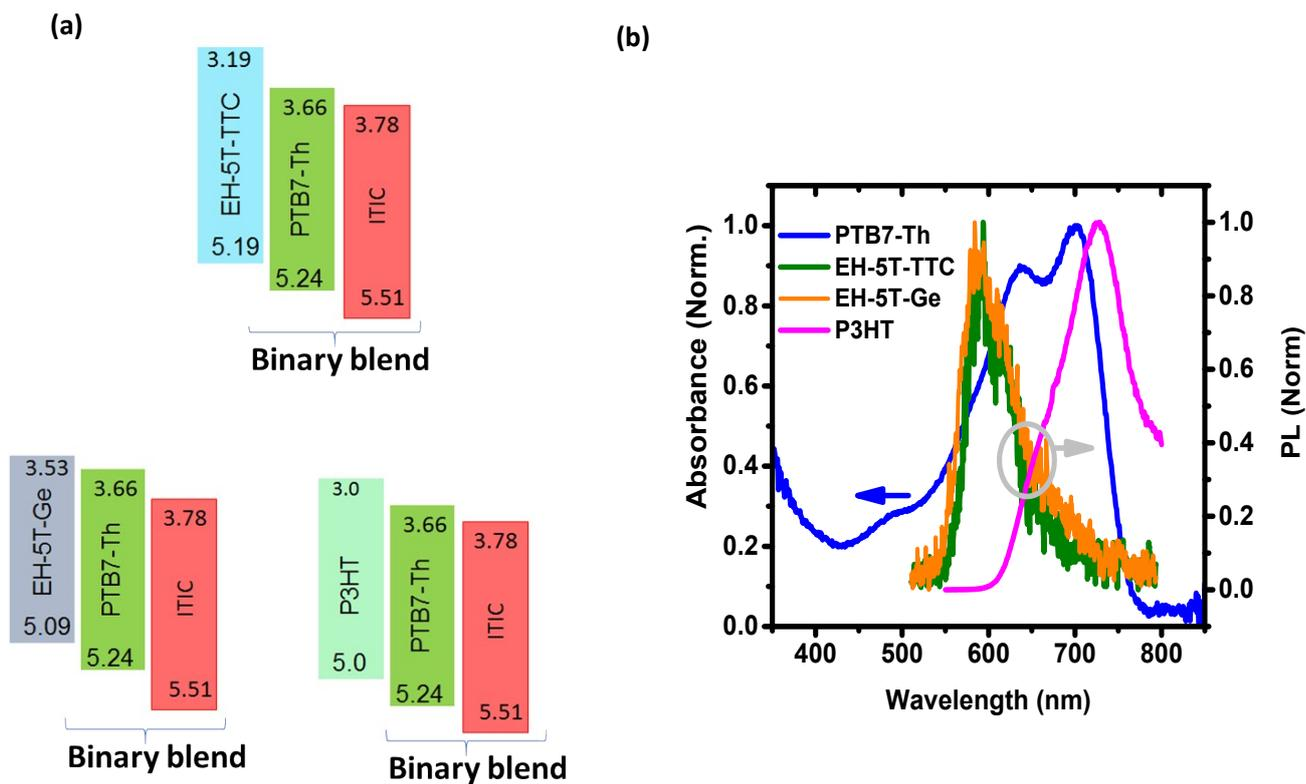
**Figure S1.** (a) Energy level diagram of the binary blend components and the ternary components. (b) The spectral overlap between the UV-Vis absorption spectra of **PTB7-Th** and the photoluminescence spectra of the ternary donor components.
