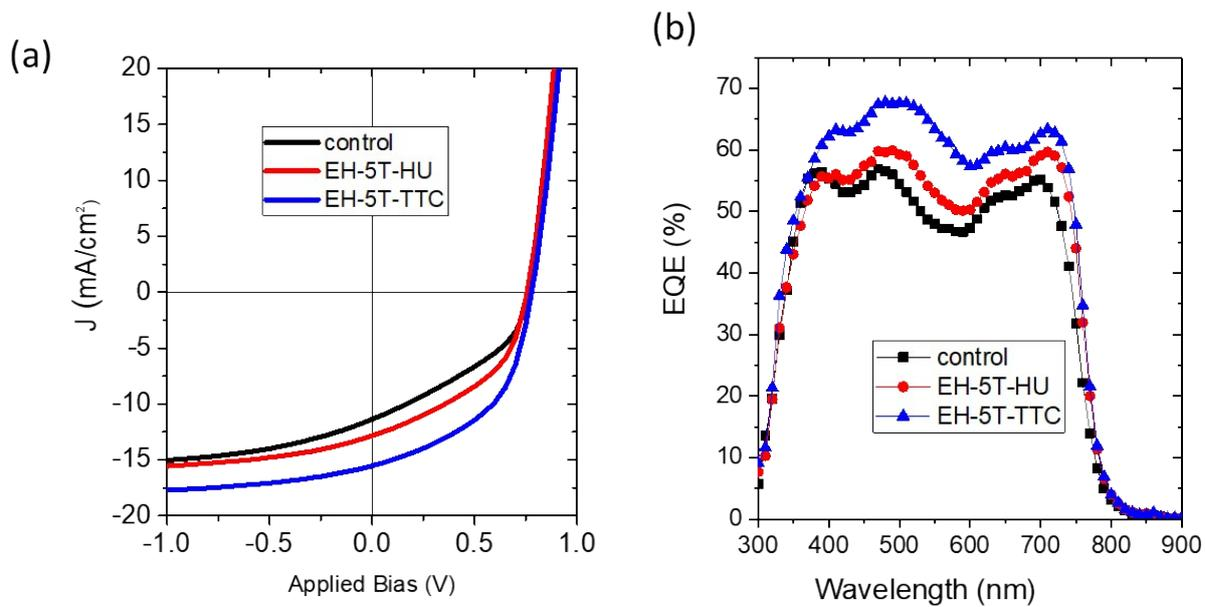
**Figure S11:** Photovoltaic performance parameters of the binary **PTB7-Th:PC<sub>71</sub>BM** and ternary blend systems using **EH-5T-HU** and **EH-5T-TTC**.
