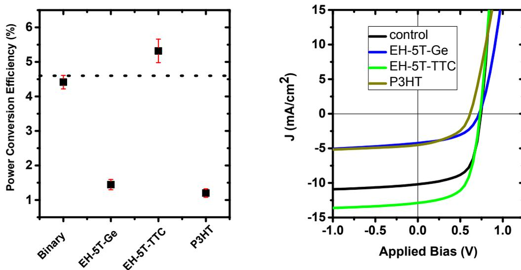
**Figure S2.** (a) Comparison of PCE and (b) J-V characteristics of the of binary **PTB7-Th:ITIC** and ternary blend systems.
