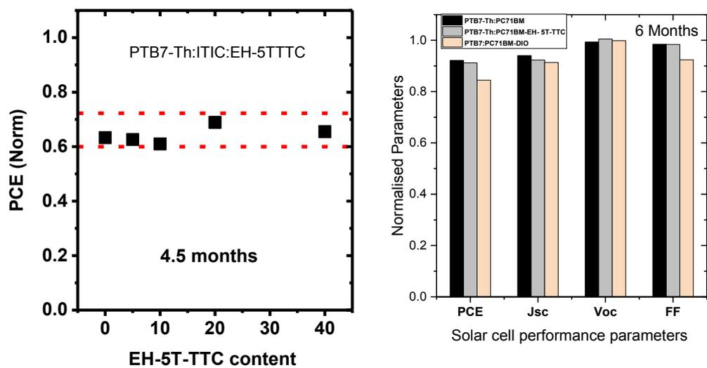
**Figure S12.** Shelf life of encapsulated ternary and binary solar cells under ambient conditions
