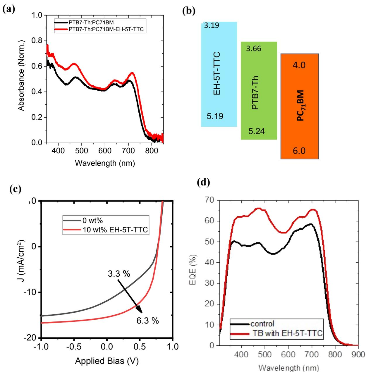
**Figure S4.** (a) Absorption spectra of the binary **PTB7-Th:PC<sub>71</sub>BM** and ternary **PTB7-Th:PC<sub>71</sub>BM:EH-5T-TTC**; (b) energy level diagram of the three components in the blend system; (c)  $J$ - $V$  characteristics of the best ternary OPV devices; (d) the EQE spectra of the binary and ternary blend systems compared.
