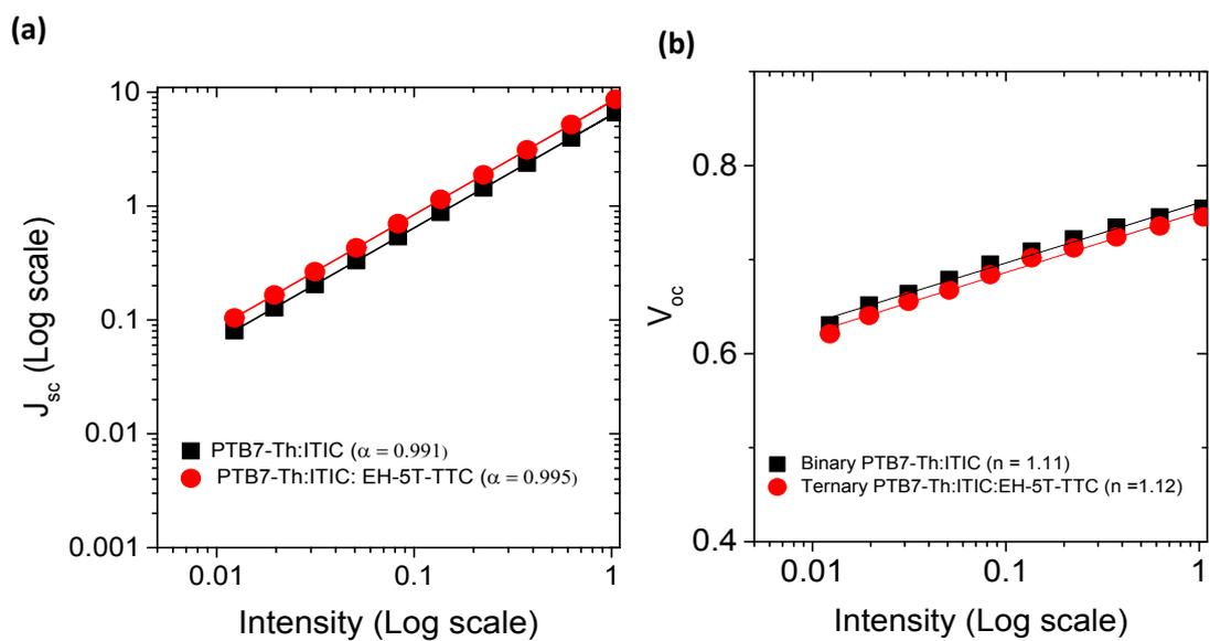
**Figure S6.** Variation of (a)  $J_{sc}$  and (b)  $V_{oc}$  as a function of light intensity for binary **PTB7-Th:ITIC** blend and **EH-5T-TTC: PTB7-Th: ITIC** ternary blend.
