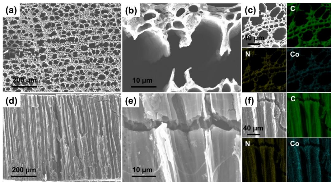
**Fig. S11** (a, b) Top-view SEM images of Co@N-HPMC after OER stability test and (c) corresponding EDX elemental maps. (d, e) Side-view SEM images of Co@N-HPMC after OER stability test and (f) corresponding EDX elemental maps.
