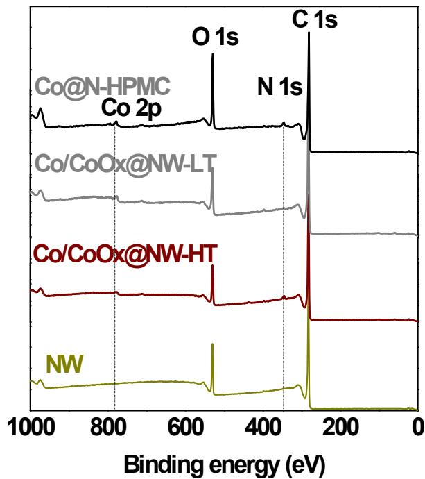
**Fig. S4** XPS spectra of NW, Co/CoO<sub>x</sub>@NW-HT, Co/CoO<sub>x</sub>@NW-LT, and Co@N-HPMC.
