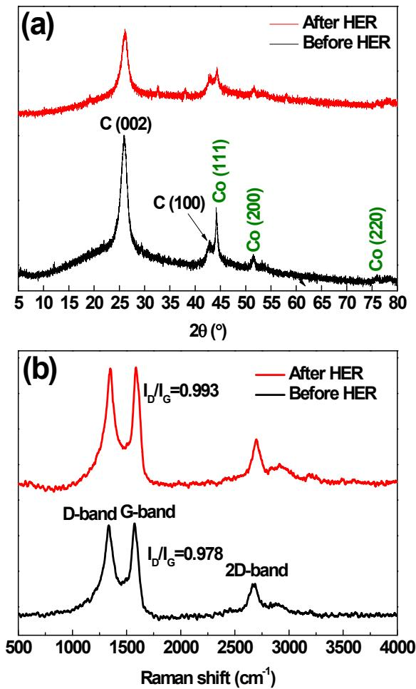
**Fig. S9** (a) XRD patterns and (b) Raman spectra of Co@N-HPMC before and after HER stability test.
