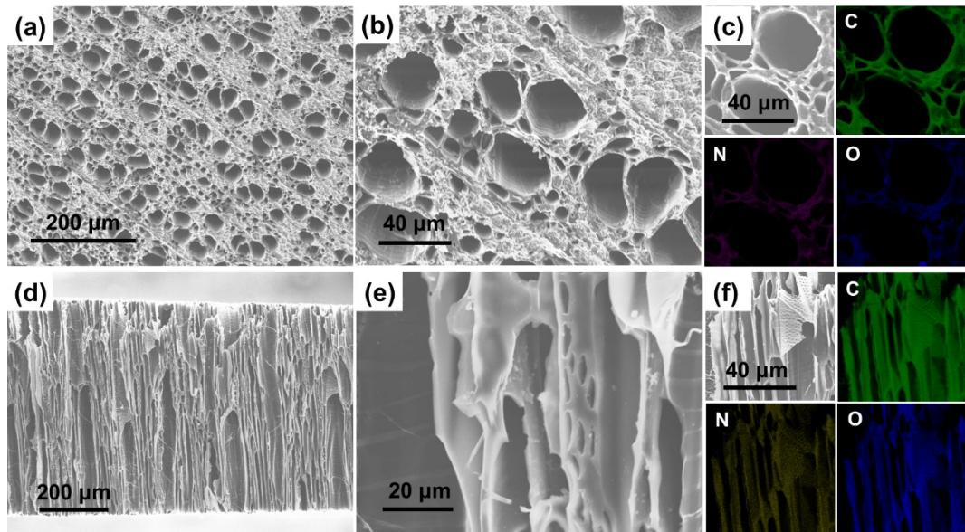
**Fig. S5** (a, b) Top-view SEM images of N-HPMC and (c) corresponding EDX elemental maps. (d, e) Side-view SEM images of N-HPMC and (f) corresponding EDX elemental maps.
