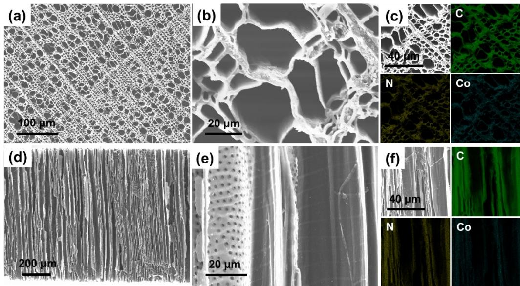
**Fig. S8** (a, b) Top-view SEM images of Co@N-HPMC after HER stability test and (c) corresponding EDX elemental maps. (d, e) Side-view SEM images of Co@N-HPMC after HER stability test and (f) corresponding EDX elemental maps.
