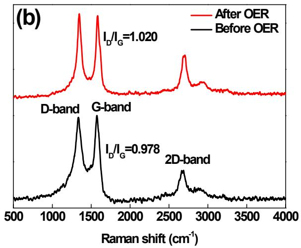
**Fig. S13** (a) XRD patterns and (b) Raman spectra of Co@N-HPMC before and after OER stability test.
