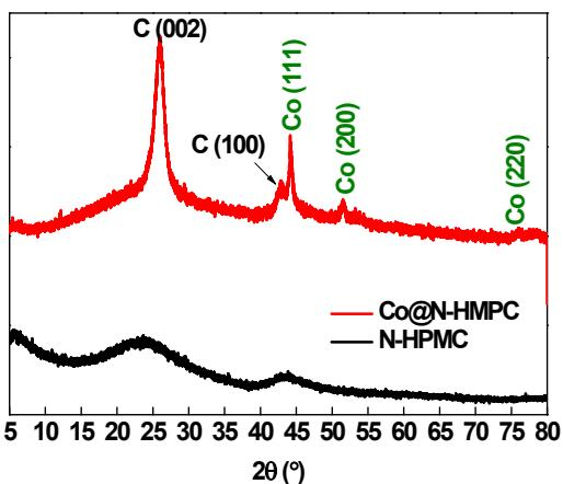
**Fig. S2** XRD patterns of Co@N-HPMC and N-HPMC.
