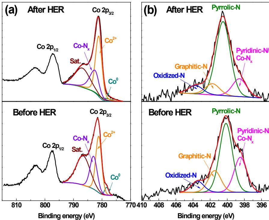
**Fig. S10** High-resolution XPS spectra of (a) Co 2p and (b) N 1s for Co@N-HPMC before and after HER stability test.
