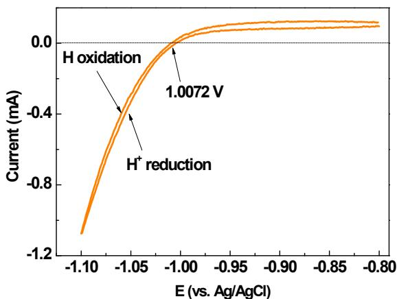
**Fig. S1** The cyclic voltammograms (CV) of Pt wire working electrode in the high purity hydrogen saturated 1 M KOH electrolyte solution. The CV scans were run at a scan rate of 5 mV s<sup>-1</sup>, and the average of the two potentials at which the current crossed zero was taken to be the thermodynamic potential for the hydrogen electrode reactions.
