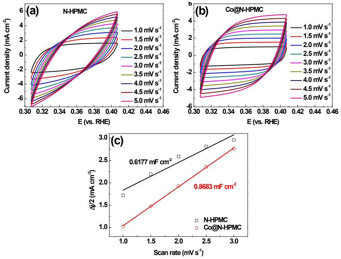
**Fig. S7** CV curves of the (a) N-HPMC and (b) Co@N-HPMC at various scan rates. (c) Comparison of  $C_{dl}$  for N-HPMC and Co@N-HPMC.
