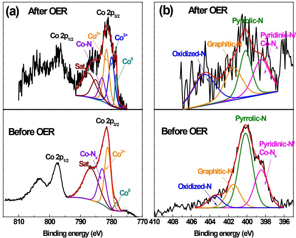
**Fig. S14** High-resolution XPS spectra of (a) Co 2p and (b) N 1s for Co@N-HPMC before and after OER stability test.
