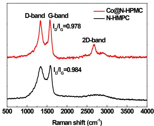
**Fig. S3** Raman spectra of Co@N-HPMC and N-HPMC.
