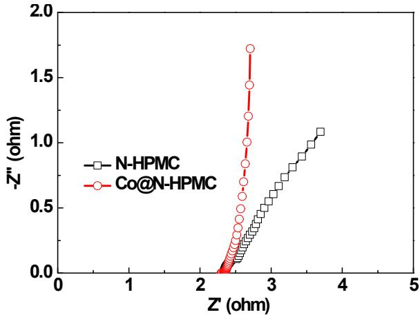
**Fig. S6** Nyquist plots of N-HPMC and Co@N-HPMC recorded in 1.0 M KOH at open circuit potential. The N-HPMC has a small semicircles in the low-frequency range of the Nyquist plots than Co@N-HPMC, indicating that the charge-transfer-related resistance ( $R_{ct}$ ) of N-HPMC is smaller than Co@N-HPMC, which is due to the fact that the presence of surface oxides on Co nanoparticles will interrupt the electron transfer within N-HPMC matrix.
